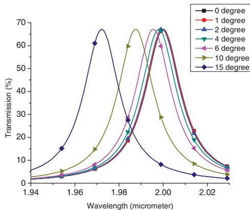
Fig. 3. Simulated transmission through the LVOF structure at different angles.
