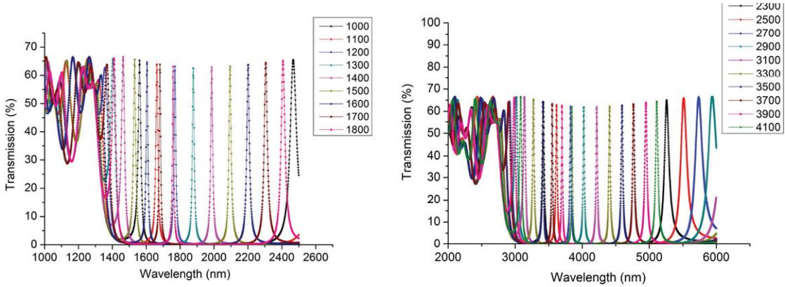
Fig. 1. (a) Transmission spectrum of IR LVOF in table 1 for different values of the cavity thickness, values in nm. (b) Transmission spectrum of IR LVOF in table 2 for different values of the cavity thickness, values in nm.
