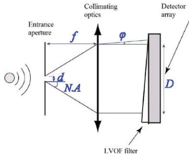
Fig. 1. Schematic of a LVOF-microspectrometer.
