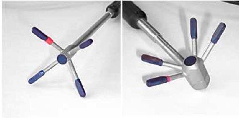
Figure (4 - 10): Downlooking probe (left) and sidelooking probe (right)
