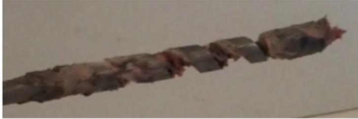
Figure 5.10: Tissue morcellated with MITE (see appendix B); tissue is clinging to the auger, resulting in inefficient automated tissue transport.
