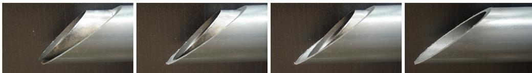
Figure 6.1: Outer sheath designed to slide respective to the vibrating inner blade. Due to the difference in angle of the tips, a variable cutting edge can be created to facilitate the motor peeling principle in various degrees.
