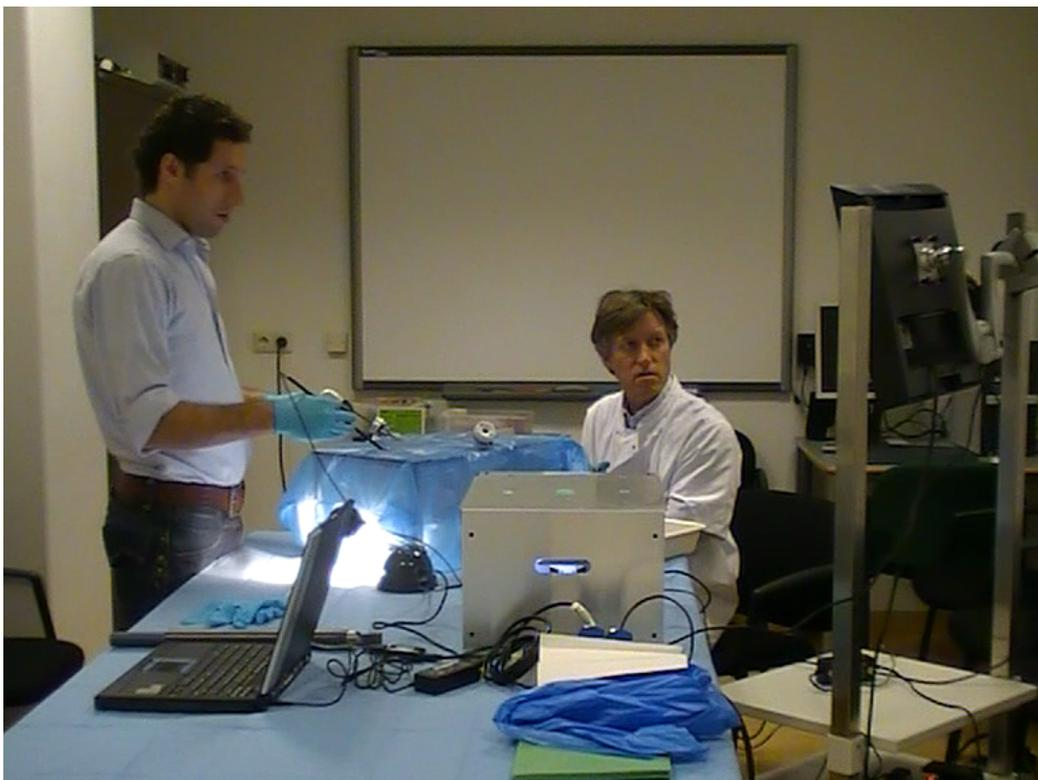
Figure 7.2: Prototype test setup with an experienced gynaecologist handling the instrument and a doctor in training (dutch: AIOSKO - Arts In Opleiding tot Specialist en Klinisch Onderzoeker) using laparoscopic graspers to present the tissue mass to the surgeon.
