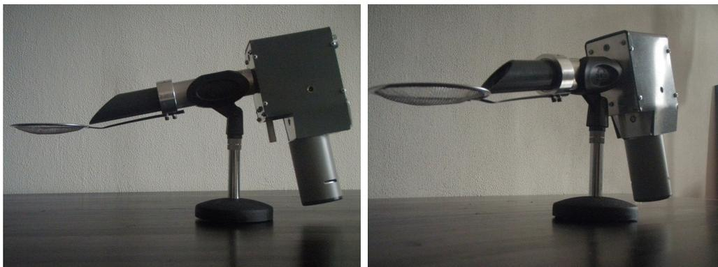
Figure 8.1: Addition for the laparoscopic test setup: trans-vaginal morcellator application simulation and shallow container cup for tissue mass at tip of morcellator.
