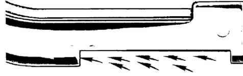
Figure 2.21: Hydrocision. Working principle: waterjet morcellation [12].
