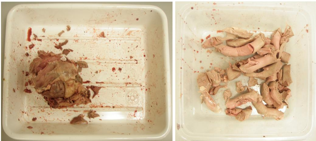
Figure 4.10: Morcellation test 6, performed by gynaecologist 1. Left: morcellated tissue mass and tissue spread (m=497g before morcellation); Right: removed tissue strips (n=37, m=101g).
