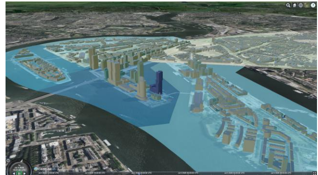
Figure 5. Example of specific cooling demand results presented at building level and annual values presented at urban function level from the study area in Rotterdam.
