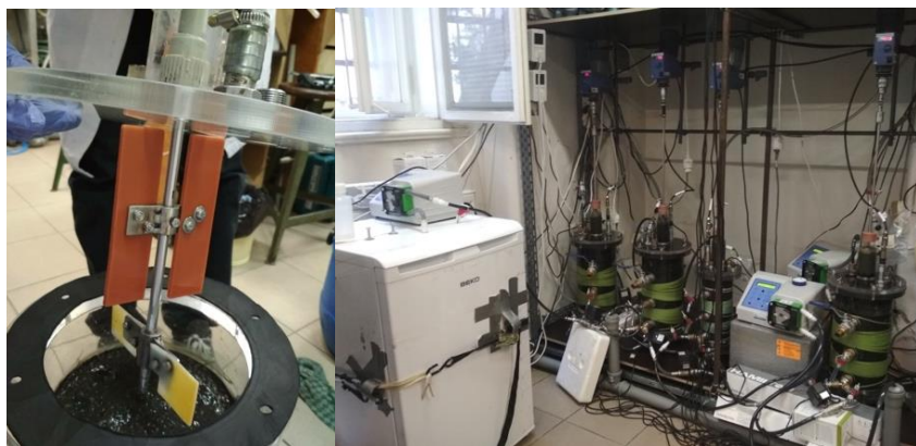
Figure 2. The lab installation: a – a new mixing system in all four reactors; b – the whole lab installation of three AD systems
