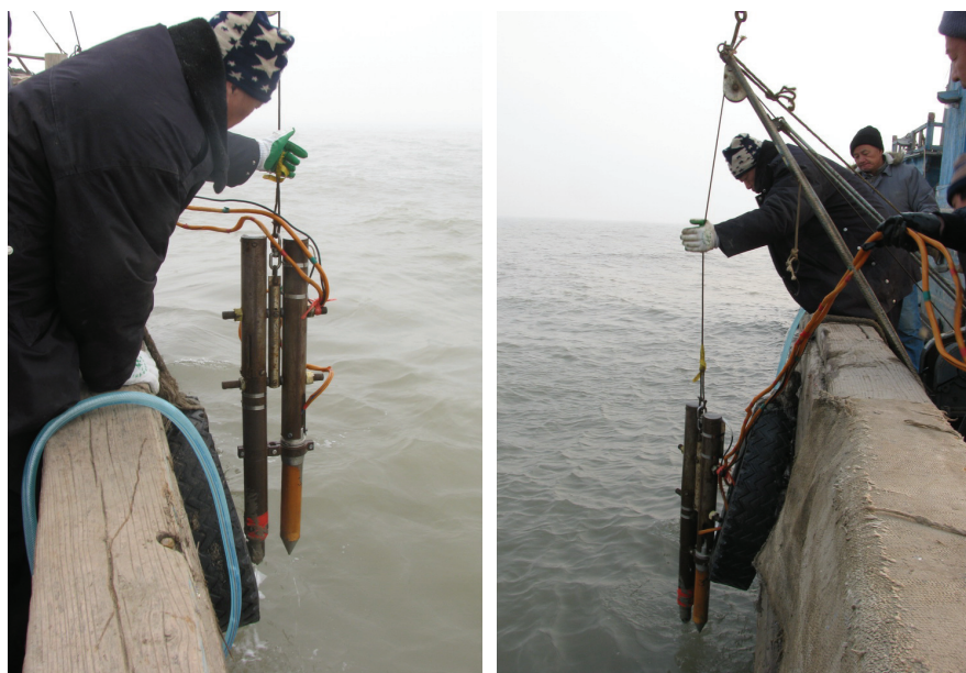
Figure 2-15. The \gamma -ray densitometer and measurement process
