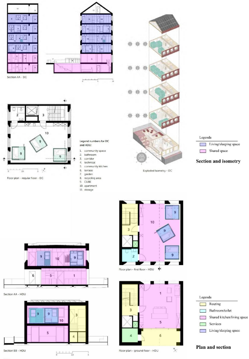
Figure 1. Local+ case study analysis project plans, sections and isometric view (Meurers, n.d.)
