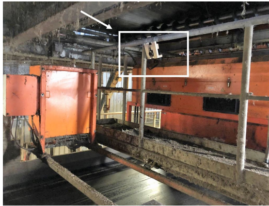
Figure 3.9: Camera above the belt
