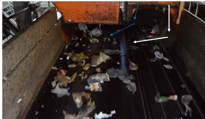
Figure 5.1: Deposition of material on the acceleration belt.
