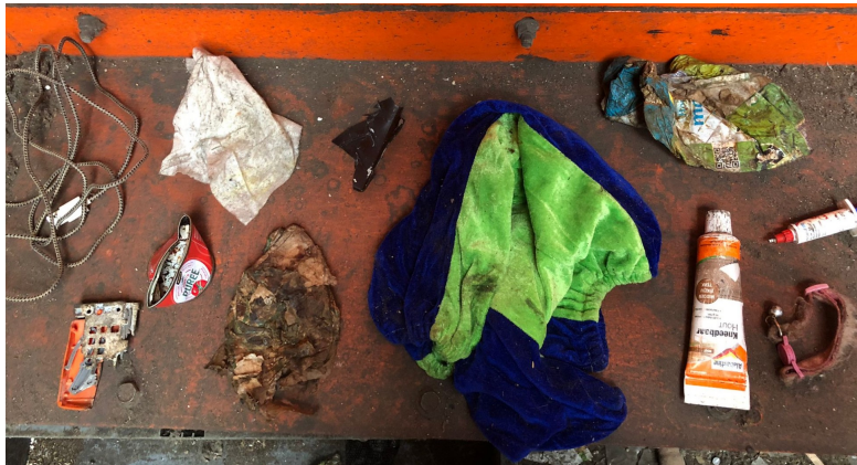
Figure 3.14: Deterministic particles found in the plastic product.
