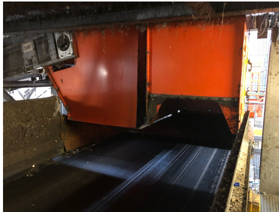
Figure 3.2: Feeding mechanism: two chutes drop material on to the belt.
