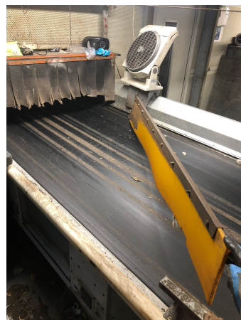
(a) Sampling location of the drop fraction: the manual sorting belt.
