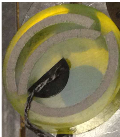
Figure 3.2: Sample for SEM-EDS microanalysis (polished section coated with carbon)
