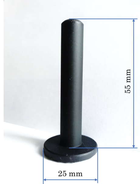
Figure 4.6: Close-up of a 3D-printed bolt
