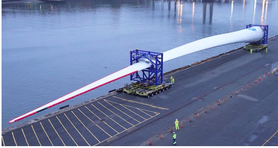
Figure 2.1: Haliade-X 12MW 108 meters blade from manufacturer GE renewable energy [23]
