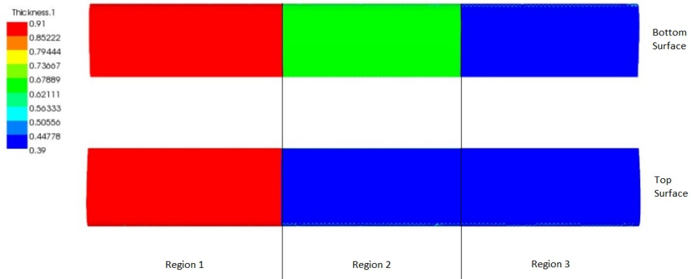
Figure 3.2: Wing thickness distribution (mm) [78]
