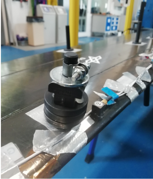
Figure 4.5: Close-up of a mass-simulated damage
