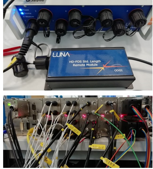
Figure 3.6: Top: the LUNA® mainframe and remote module. Bottom: the imc® mainframe
