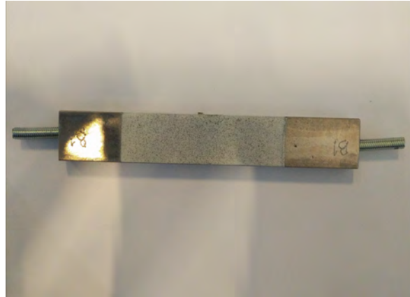
Figure 3-8: Speckle pattern produced from paint sprays for DIC.
