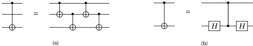
Figure A.1: Distributed CNOT operation (a) and a CNOT gate rewritten in terms of two Hadamard gates and a CZ gate (b).
