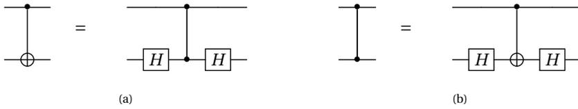
Figure 2.8: CNOT gate rewritten in terms of a CZ gate and two  $H$  gates on the target qubit (a) and vice versa (b).
