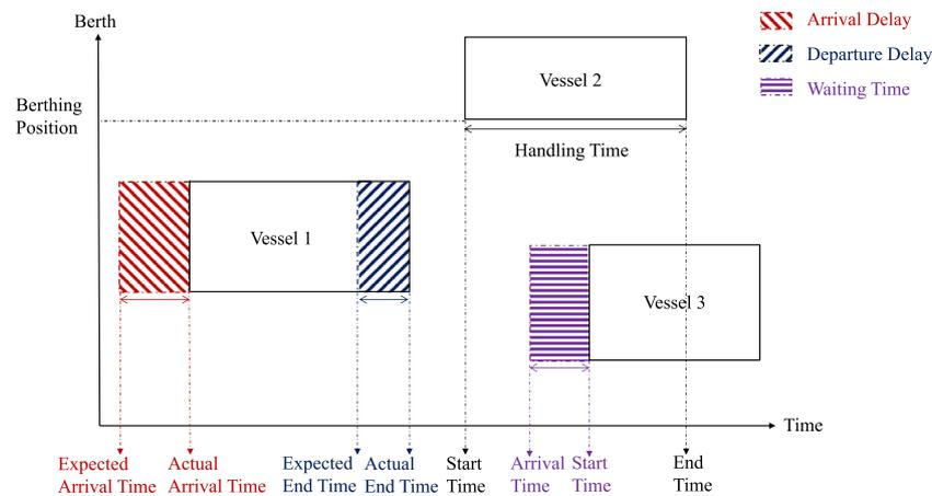
Fig. 1. An illustration of the two-dimensional berthing plan.
