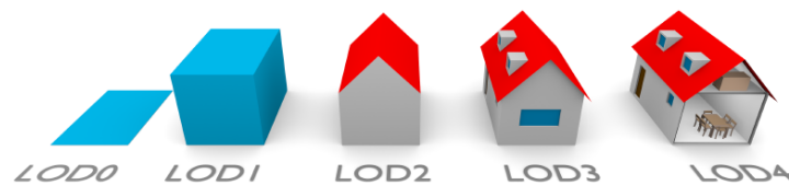
Figure 2.8: LOD in CityGML [Biljecki et al., 2017].
