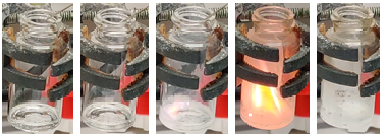
Figure 5.4: The reaction between 97% HTP and 1.0M TEA solution in hexanes in open air. Frame 1 : reaction vessel filled with 97% HTP. Frame 2 : white fumes as TEA solution is added. Frame 3 : start of ignition. Frame 4 : full combustion. Frame 5 : leftover aluminum oxide from the reaction.
