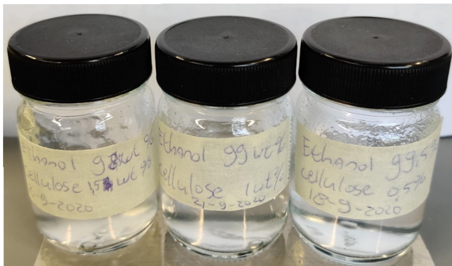
Figure 3.3: Samples created by mixing ethanol with 1.5%, 1%, and 0.5% thickening agent.
