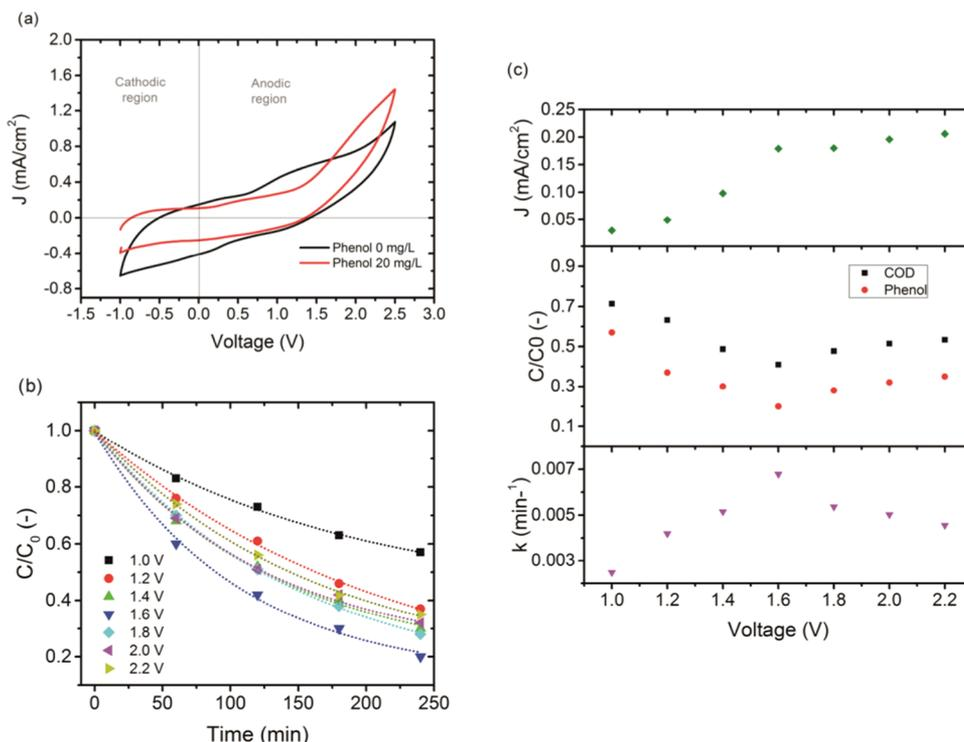
**Figure 2.** Characteristics of a graphite/graphite electrochemical system connected to a voltage source, (a) *JV* characteristics, (b) phenol degradation at different applied potentials, and (c) the corresponding first-order reaction constant; the current density measured flowing through the system at each voltage and the final concentration and COD in the sample after 4 h of degradation at different voltages.
