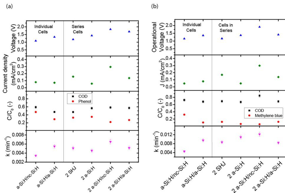
**Figure 4.** (a) Phenol and (b) methylene blue degradation characteristics when using different solar cells. The current densities reported are based on the electrode area of 16 cm<sup>2</sup>.
