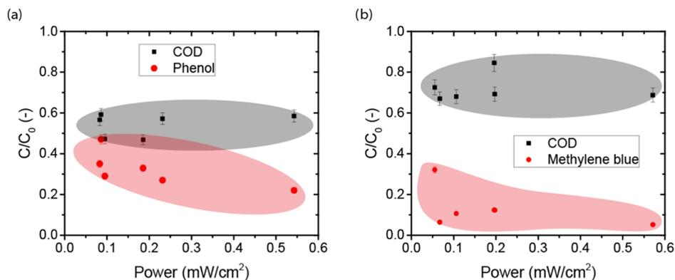
**Figure 5.** Concentration of (a) phenol and (b) methylene blue and their respective CODs after 4 h of degradation with respect to the power provided by the different solar cell configurations. The power densities refer to the areas of the electrodes, which are 16 cm<sup>2</sup> per electrode.
