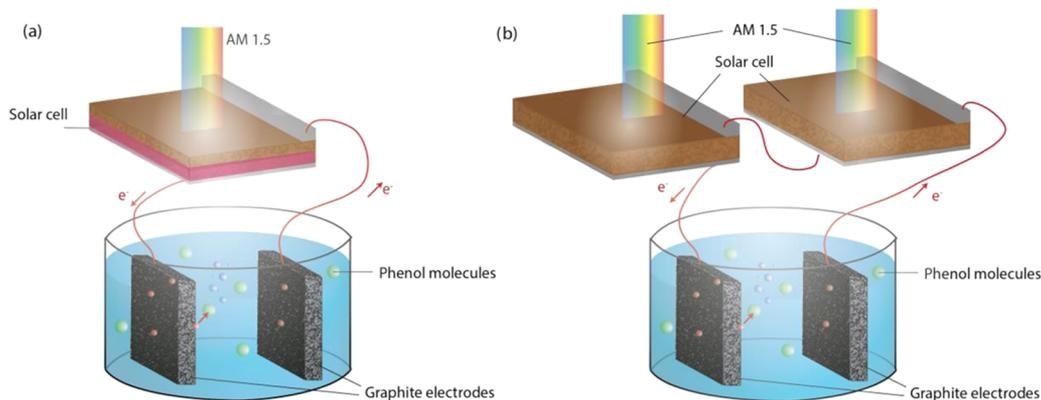
**Figure 1.** Schematic of a stand-alone device configuration combining an electrochemical system and (a) a solar cell, possibly multijunction, or (b) several solar cells connected in series, which can be either single or multijunction.
