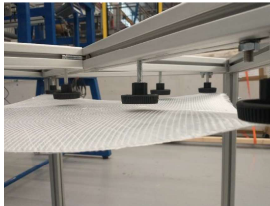
Figure 2. Frame with a 550 x 550 mm reinforcement suspended from the pick-up points
