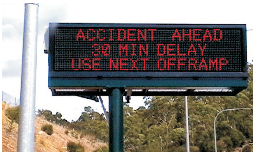
Figure 7.1: Example of VMS for incident management
