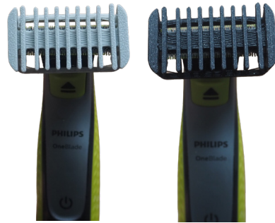
Figure 24: Final prototypes in PETG (left) and PLA (right)
