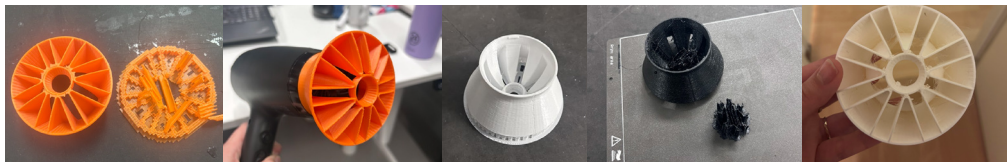
Figure 34: Prototypes to test print orientation and fit
