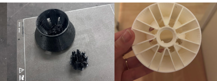
Figure 35: PETG and TPU prototypes
