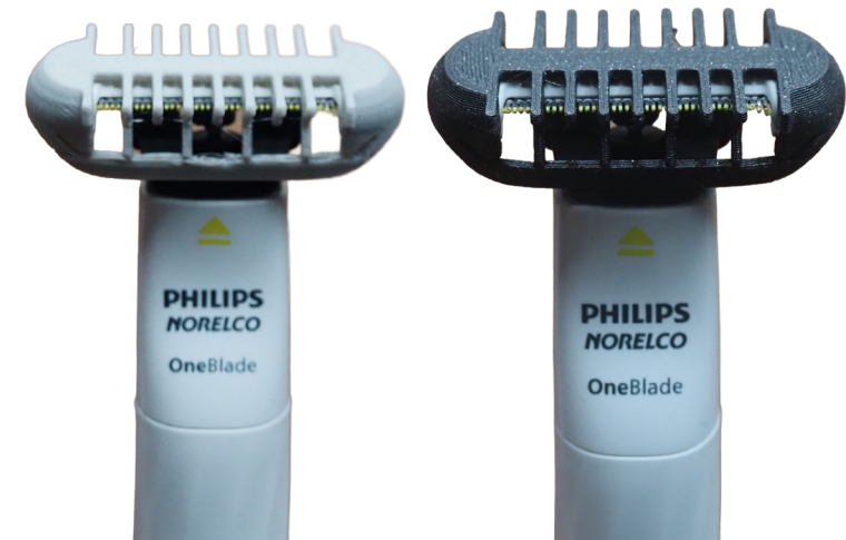
Figure 86: Final prototypes in PETG (left) and PLA (right)
