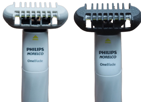
Figure 19: Final prototypes in PETG (left) and PLA (right)
