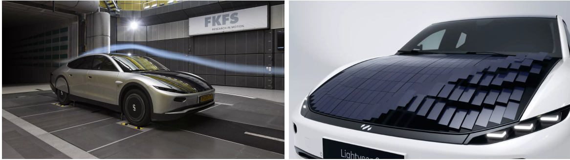
(a) Lightyear 0 is designed to minimize aerodynamic drag
