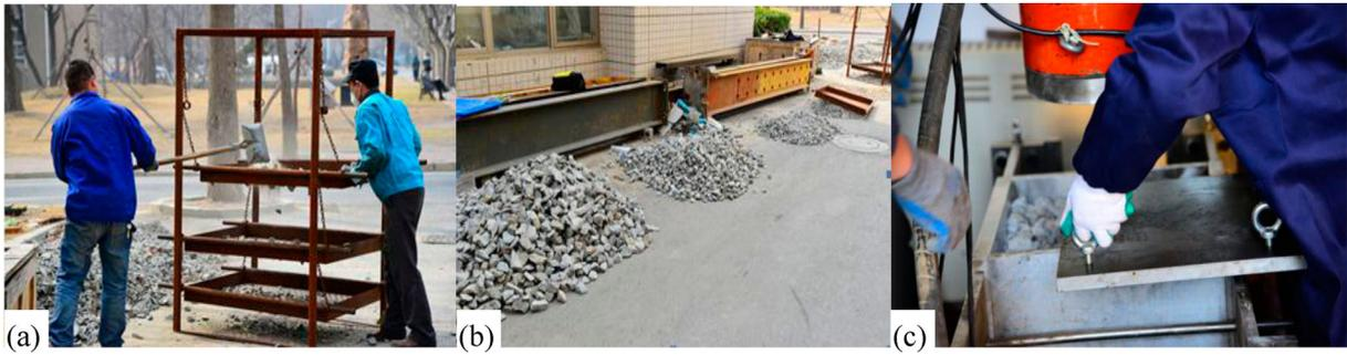
**Figure 12.** Overview of the shear test preparation: (a) screening ballast; (b) classifying ballast; (c) loading ballast.
