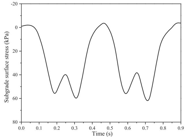
Figure 22. Simulation results of subgrade dynamic stress.
