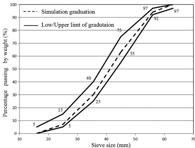
Figure 3. Particle size distribution of the ballast materials.
