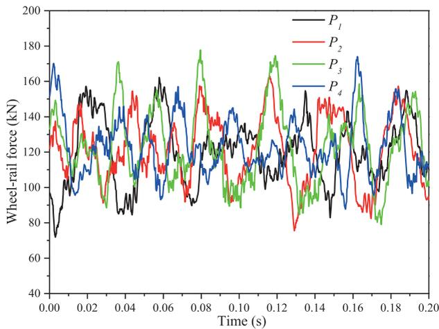
Figure 9. (Colour) Wheel-rail force curves of four wheelsets.
