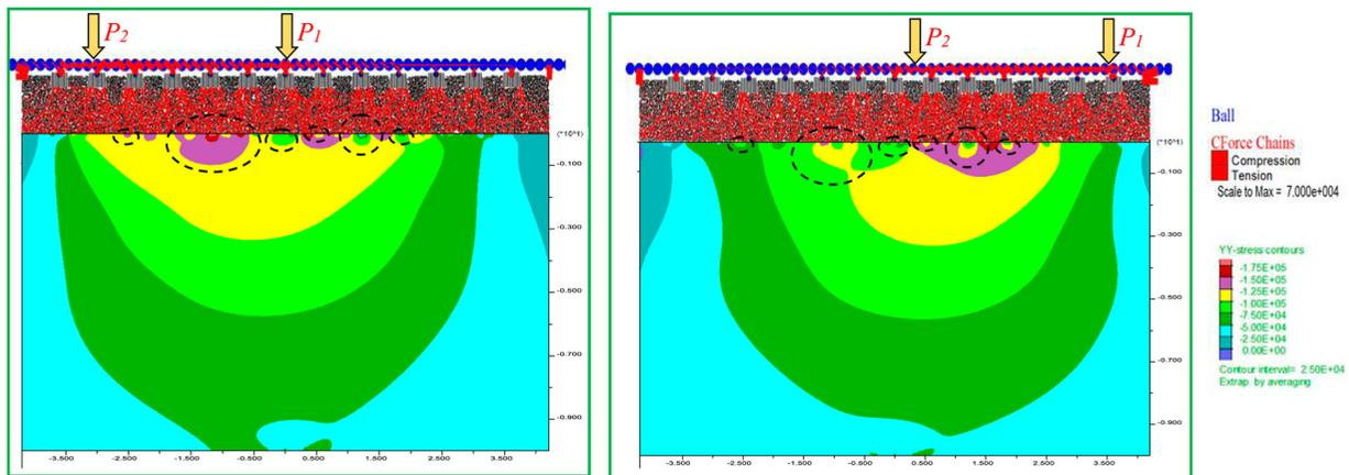
Figure 25. (Colour) The change of vertical stress contour  $\sigma_{yy}$  and contact force under moving loads.
