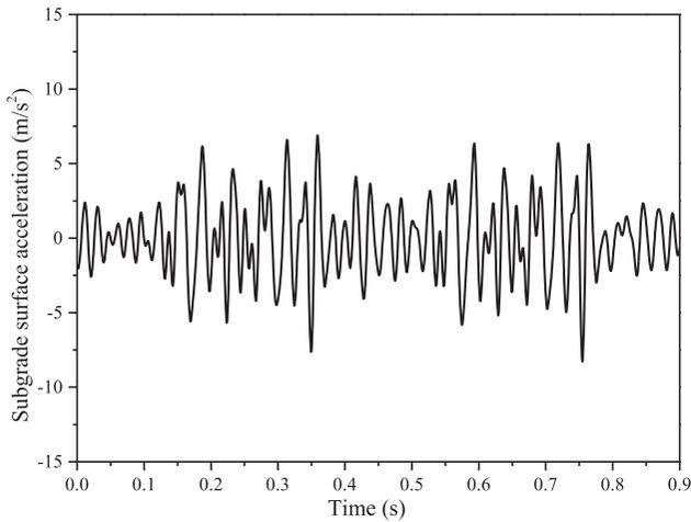
Figure 23. Simulation results of subgrade dynamic acceleration.
