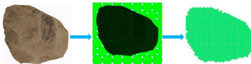
Figure 2. Simulation of the ballast with complex shape.
