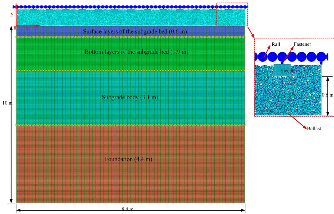
Figure 7. Coupled railway ballast track and substructure model.
