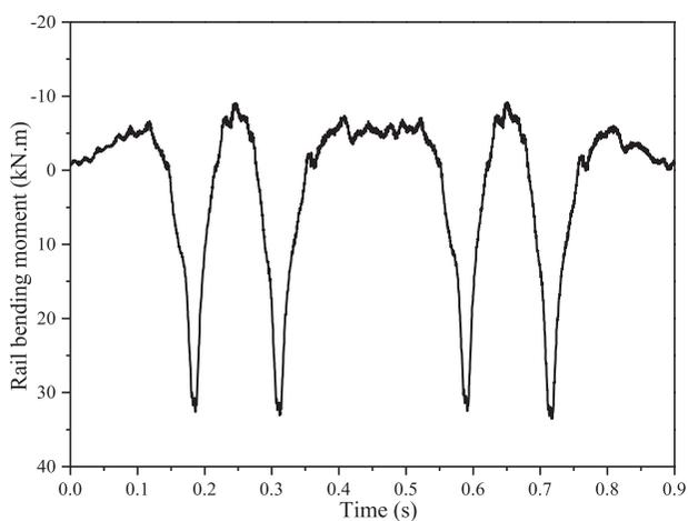
Figure 17. Simulation results of rail bending moment.
