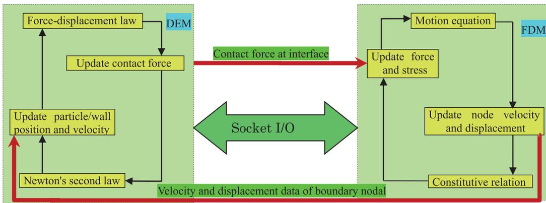
Figure 8. Flowchart of discrete-continuum coupling process.
