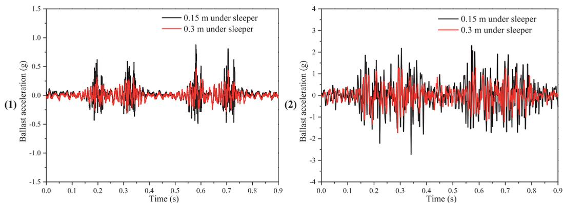
Figure 21. (Colour) Ballast acceleration results: (1) field test result; (2) simulation result.
