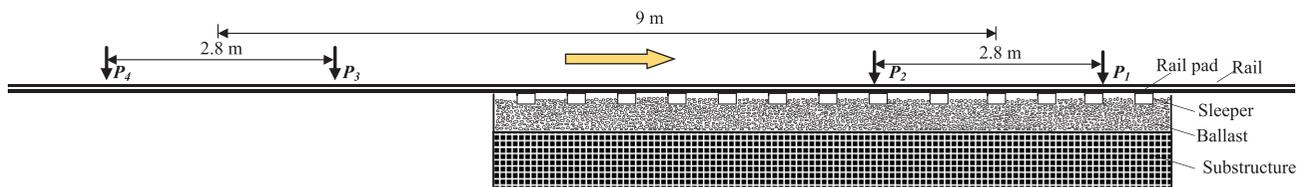
Figure 10. Schematic of wheel-rail forces applied into the coupled DEM/FDM model.
