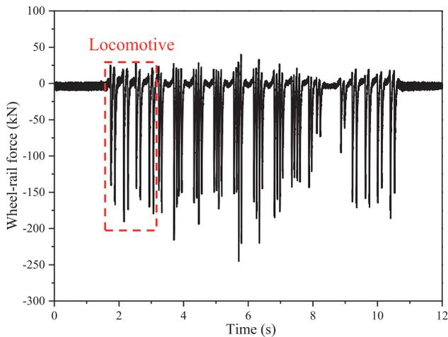
Figure 16. The measured wheel-rail force.
