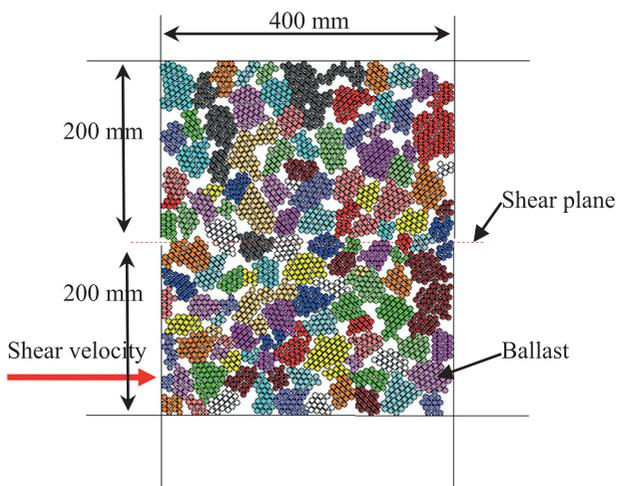
**Figure 13.** (Colour) Initial assembly of large-scale direct shear test.
