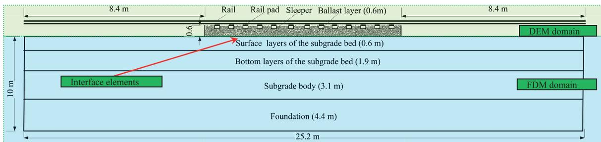
Figure 1. Longitudinal railway ballast track and substructure profiles.
