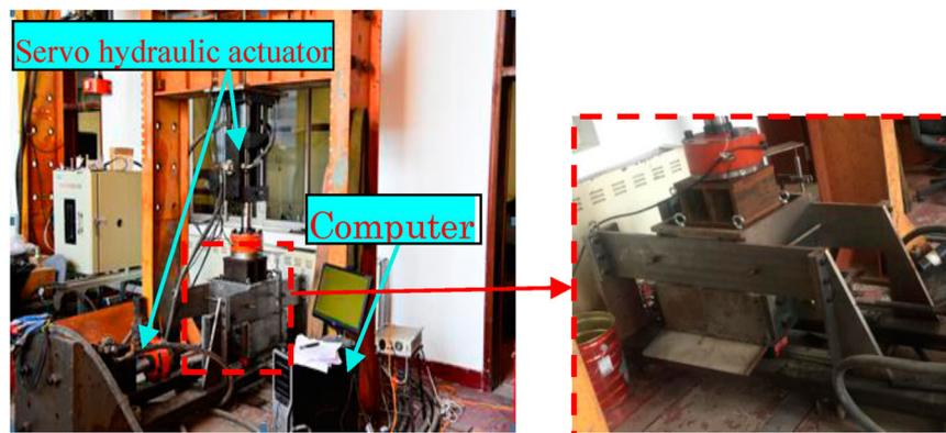
Figure 11. Direct shear test: middle-scale direct shear apparatus with upper and lower shear boxes.
