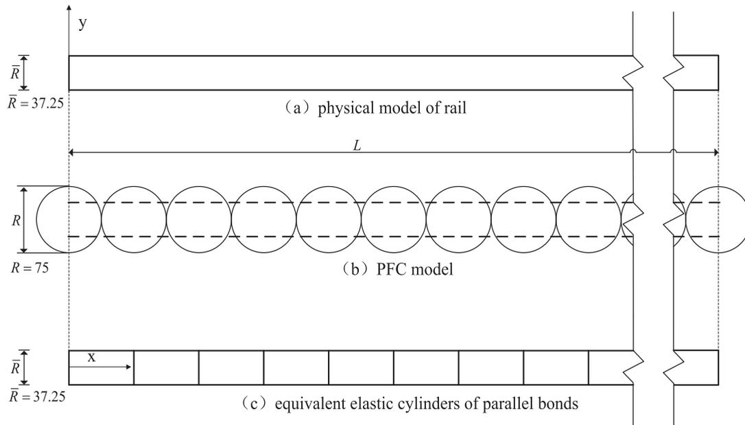
Figure 4. Simulation of the rail in PFC.
