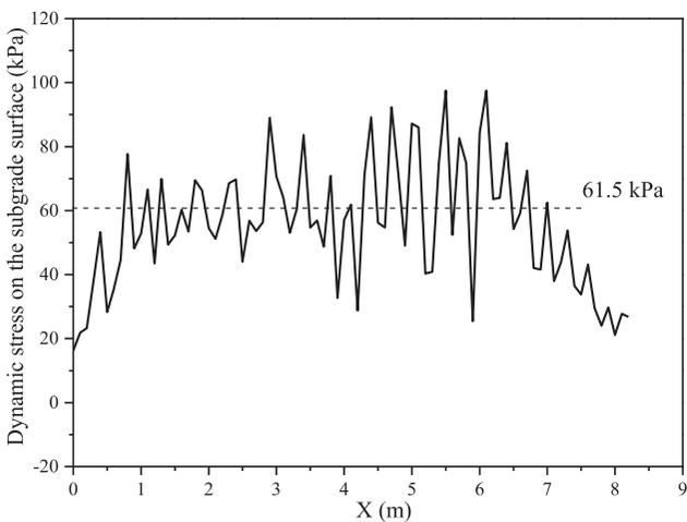
Figure 24. Longitudinal distribution of the maximum dynamic stresses on the subgrade surface.
