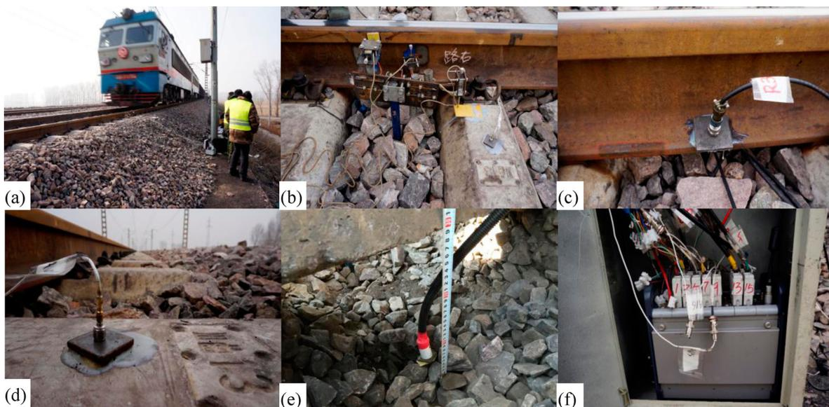
**Figure 15.** Field testing: (a) field test location; (b) displacement sensors; (c) accelerometer on rail; (d) accelerometer on sleeper; (e) accelerometer embedded in ballast layer; (f) data acquisition system.
