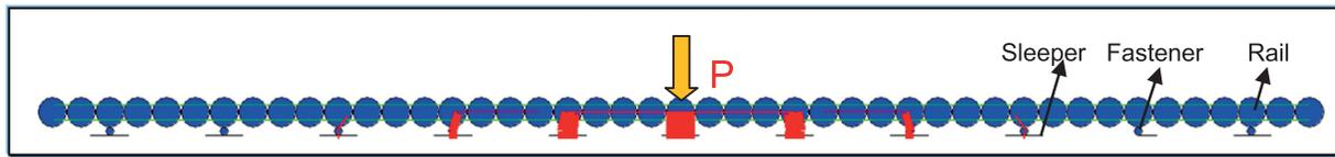
Figure 5. (Colour) Numerical test of the PFC rail model.
