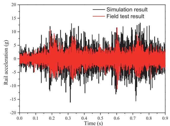
Figure 19. (Colour) Rail acceleration results.
