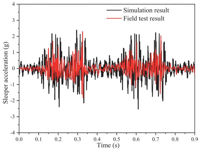
Figure 20. (Colour) Sleeper acceleration results.
