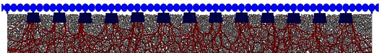
Figure 6. (Colour) The initial state of railway ballast track discrete element model.
