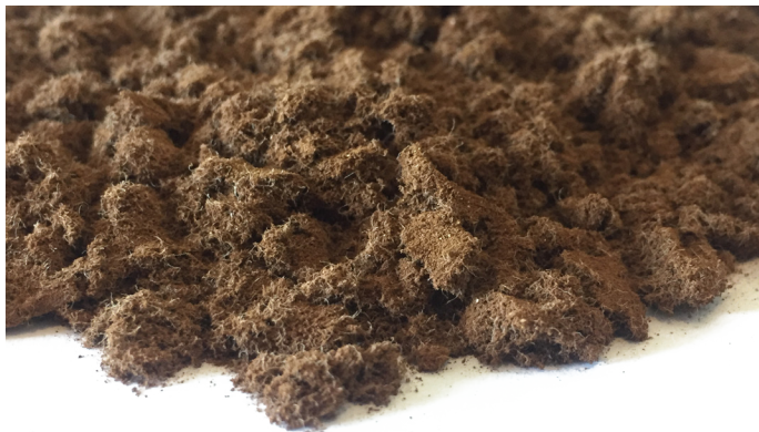
Figure 58: Product of the process, fiber reinforced lignin draped in a petri dish
