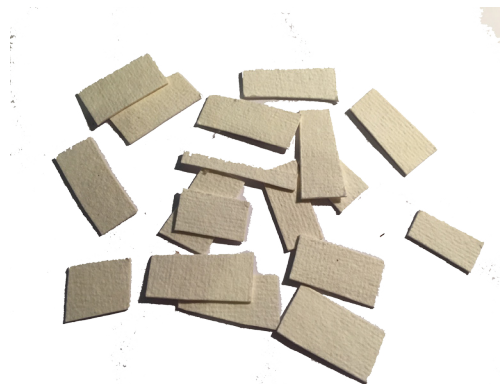
Figure 47: chips of Skogcell 90Z bleached kraft WFBR with approximate size of 25 mm x 15 mm
