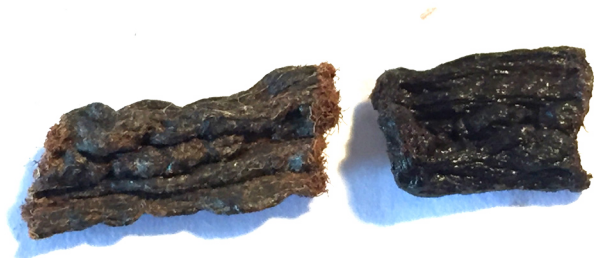
Figure 97: water test: on the left material sample of batch 9. On the right material sample of batch 9 after being wetted in water for 168 hours.
