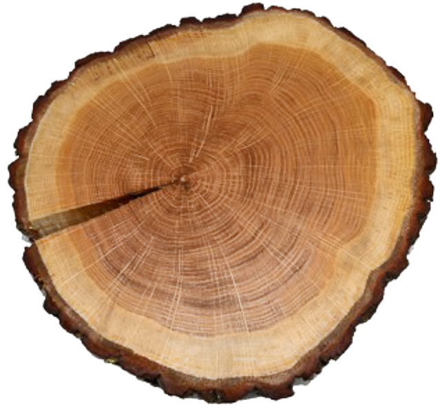
Figure 12: clear differences visible between heartwood and sapwood in this piece of oak.
