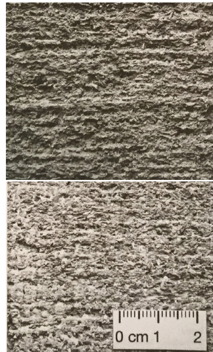
Figure 33: Inner structure of cone with bonded with cement (top) and gypsum (down) source: Henke & Treml (2012)
