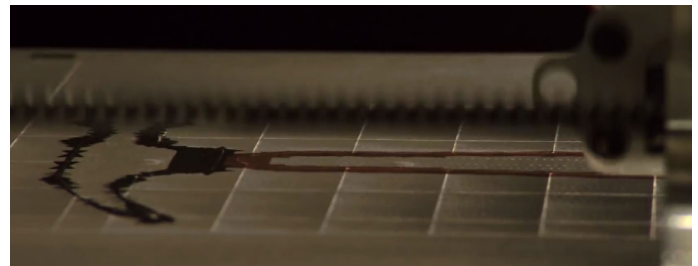
Figure 38: step 4: the machine takes a sheet and puts adhesives on it. At the location of the hammer a lot, next to it, on the excess material, less.
