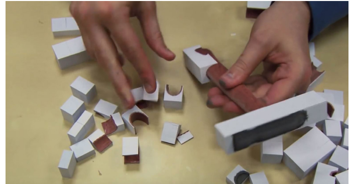
Figure 43: step 9: Now the printed object can be separated from the excess material
