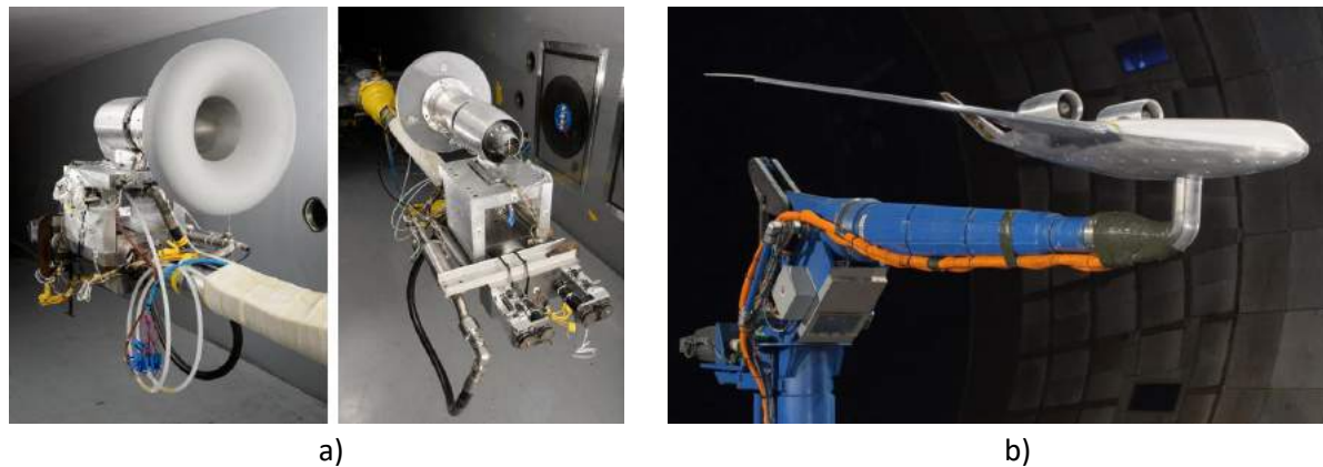
Figure 1.5: a: Static Calibration of TPS in the Wind Tunnel b: Hybrid Wing Body Wind Tunnel Model
