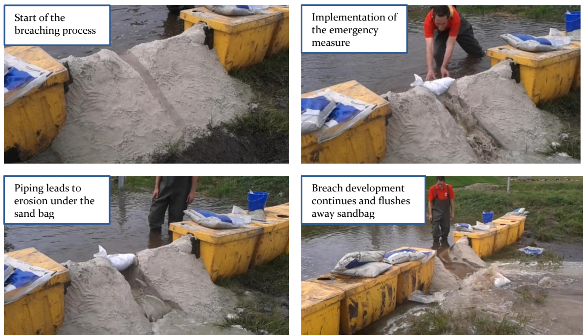
Figure 6.4: Experiment 1, snapshots are taken at t = 5 s, 40 s; 55 s and 80 s after overtopping
