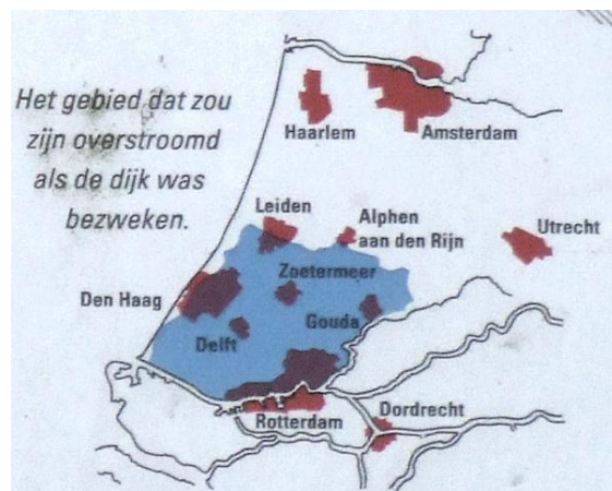
Figure 4.1: Inundated area if the dike breached 3
