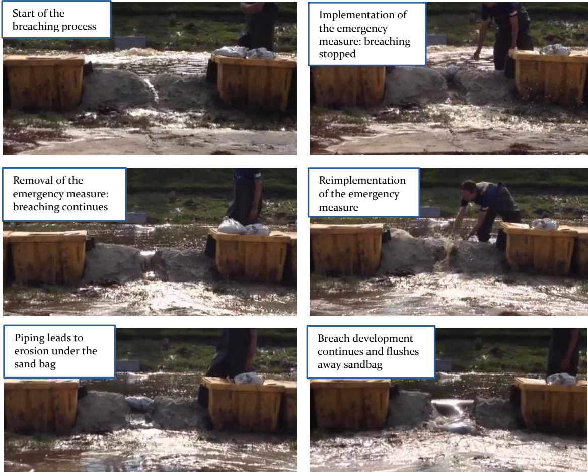
Figure 6.5: Experiment 2, snapshots are taken at t = 5 s, 30 s; 55 s, 70 s; 80 s and 95 s after overtopping
