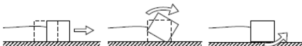
Figure 5.35: Failure mechanisms shearing, rotation and piping, (Boon, 2007)
