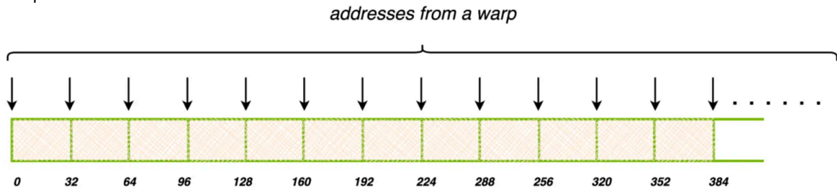
Listing 1: Uncoalesced memory access pattern showing each thread (arrow) accessing data in a separate 32-byte memory sector. Courtesy: NVIDIA Technical Blog 21 .
