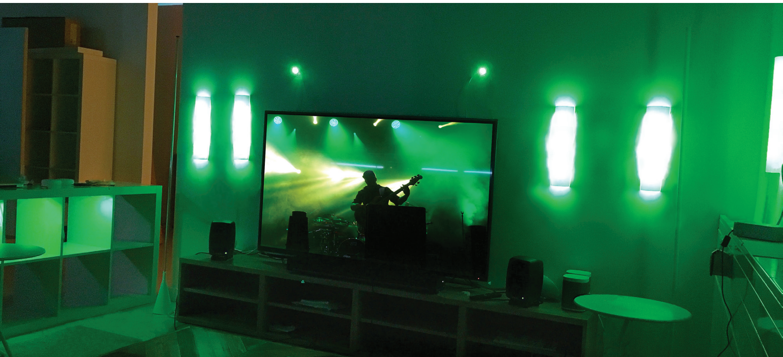
Figure 27: Final design The final design has individual lights that can be placed through a living room and sync with music.
