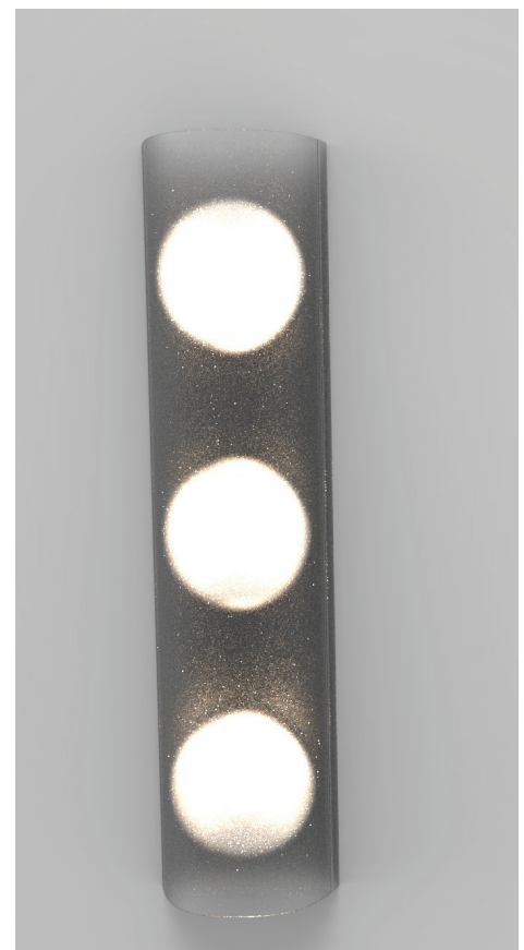
Figure 29: Collective diffusion. Three pucks together in a diffuser create a pixelated light object.
