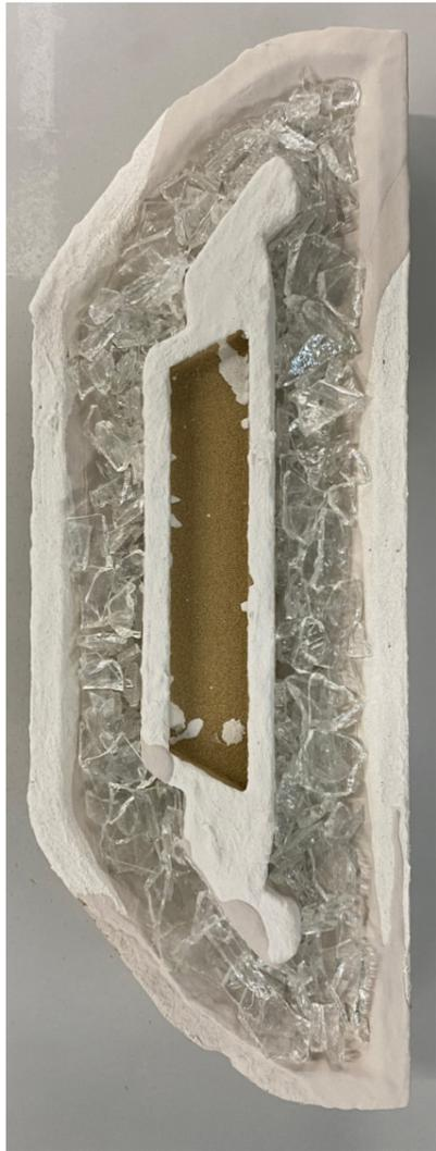
4 Mould after firing at 870°C
