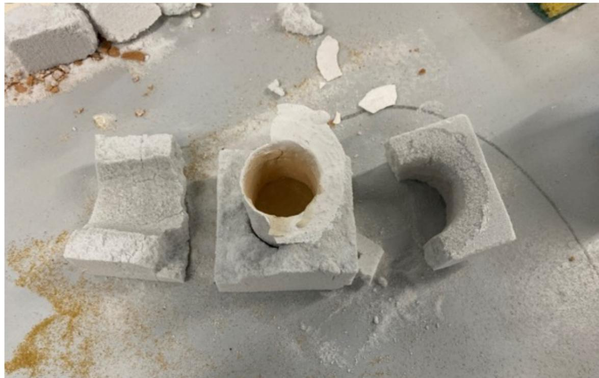
Figure 95 : Crystalcast protective layer after de-moulding from quartz sand mould.
