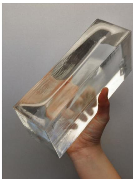
Figure 75 : Directional transparency of laminated glass as displayed in the project Glass wipe by (Eckersley O'Callaghan, 2018)
