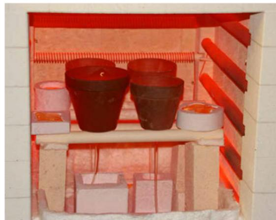
Figure 47 : Primary casting or hot pouring (top), image credits: Marcel Bilow. Secondary casting or kiln casting (bottom) (Oikonomopoulou, 2019)
