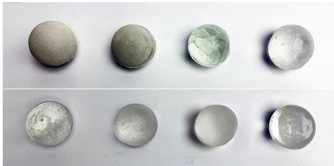
Figure 7 : experiments using different coatings, top kiln casting, bottom foundry casting (Giesecke & Dillenburger, 2022)
