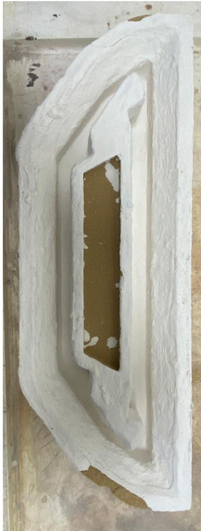
2 Coating application (Zirkofluid 6672, 2X flow). Drying of 1,5 hrs between each layer
