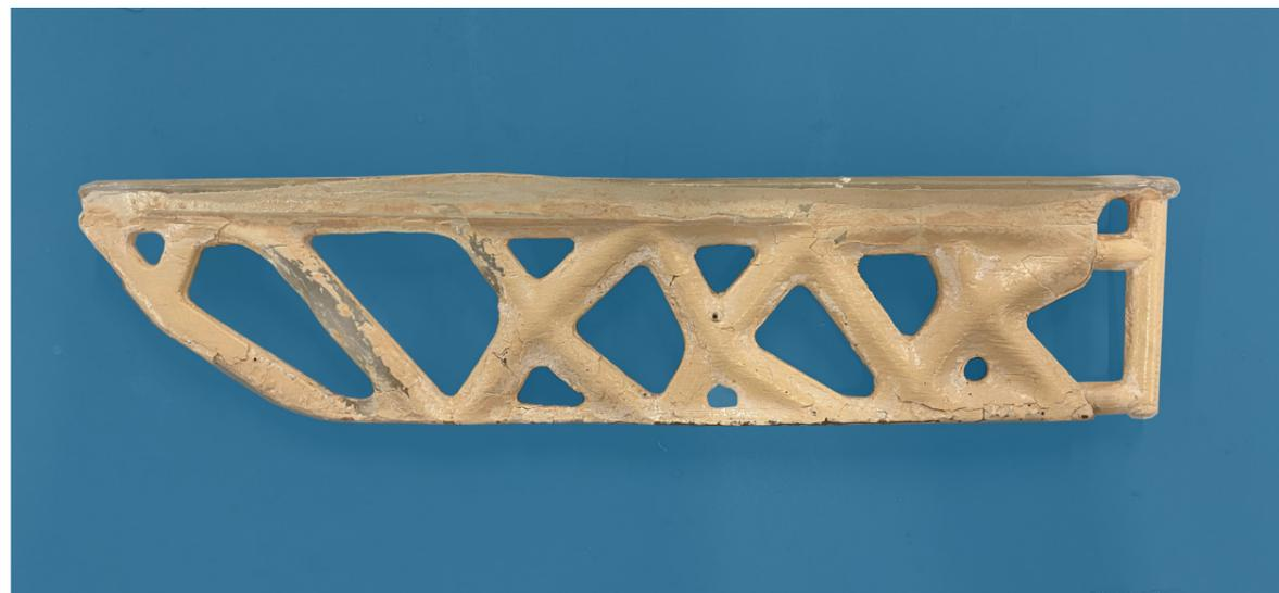
Figure 142 : Glass prototype after demoulding. Coating is attached to glass but can be cleaned relatively easy with the use of a sponge and bremel.
