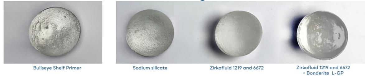
Figure 57 : The use of various coatings for glass casting on 3DPMSM , edited from (Giesecke & Dillenburger, 2022)
