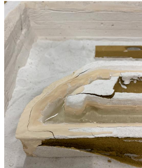
Figure 126 : Mould after firing. Some chipping of the crystalcast protective layer with a part of the sand mould.
