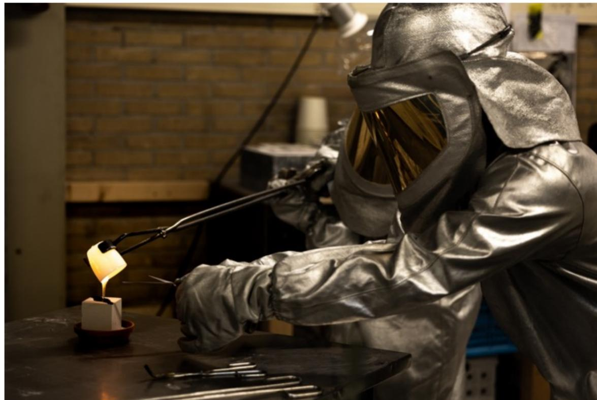
Figure 97 : Hot pouring of glass on 3DPSM, cutting of glass string, behind: Telesilla Bristogianni, front: author. Image credits: Marcel Billow
