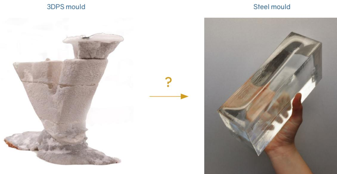
Figure 87 : Left kiln cast glass using disposable 3DPSM (Bhatia, 2019). Right foundry cast glass using steel moulds. Difference in the surface quality is evident (Oikonomopoulou, Bristogianni, Veer, et al., 2018)
