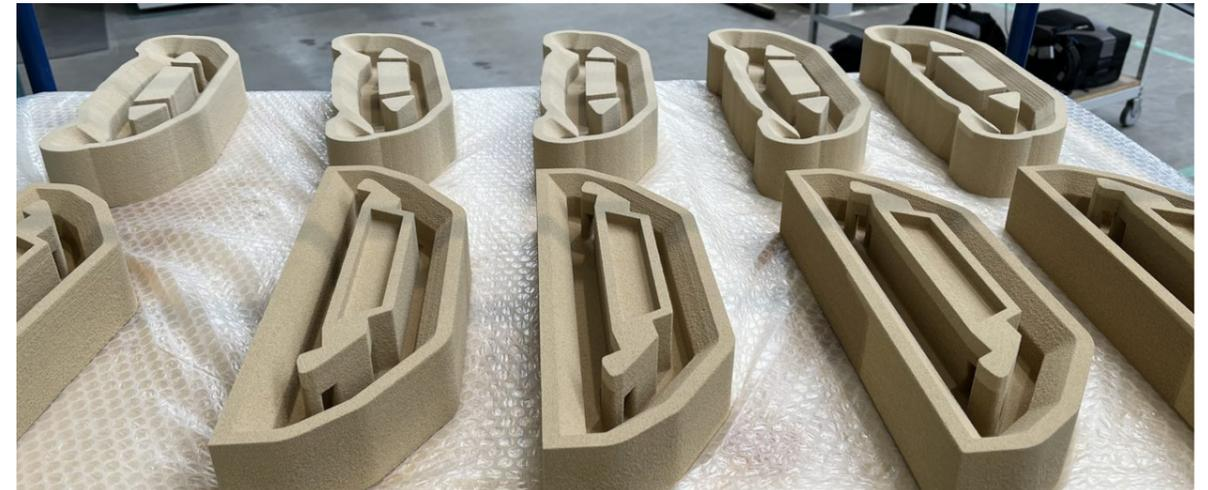
Figure 125 : Larger size moulds of TO beam geometries printed on ceramic sand with Inorganic binder, ExOne. Large dimension approx. 35 cm in length.
