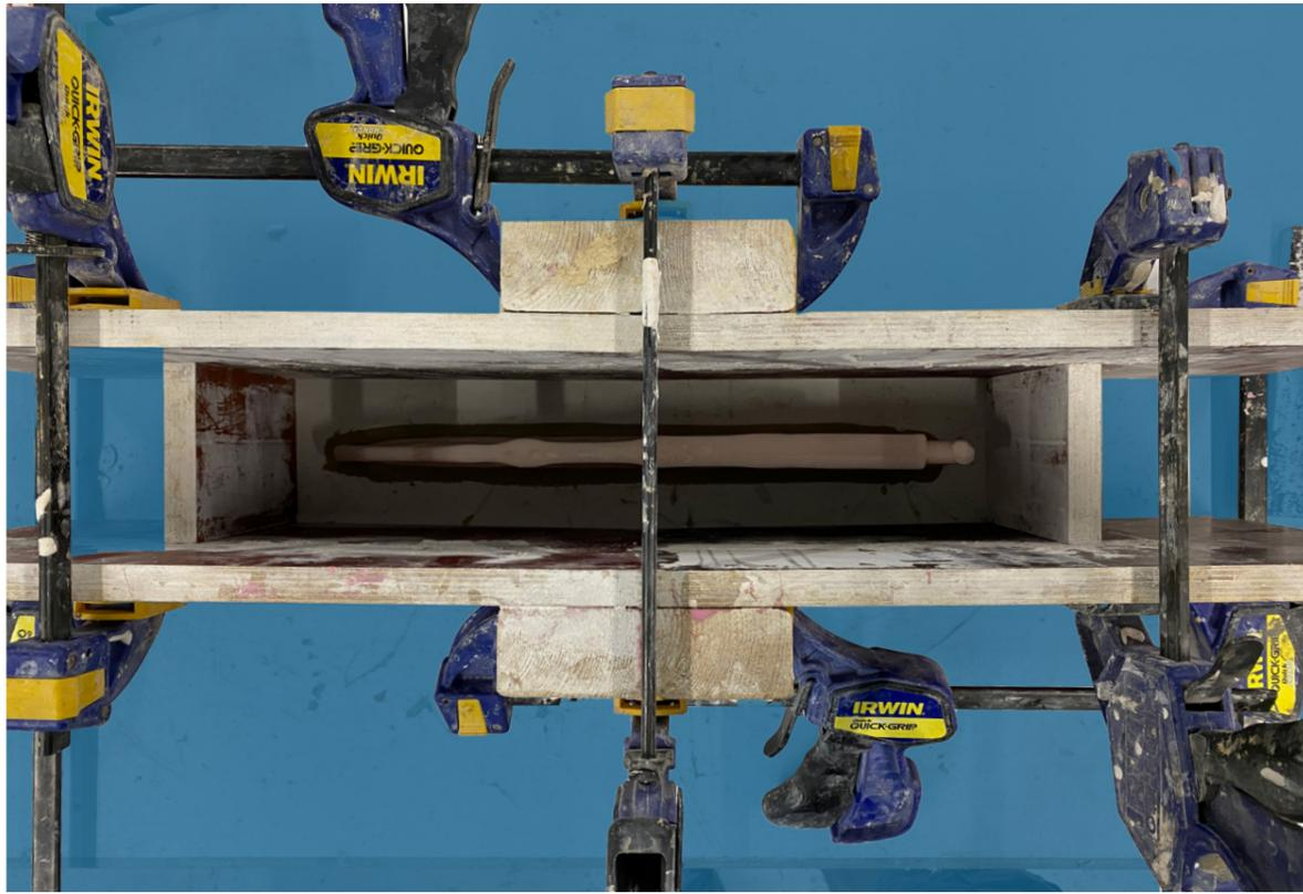
Figure 137 : Investment casting of the wax positive. Mould set up.
