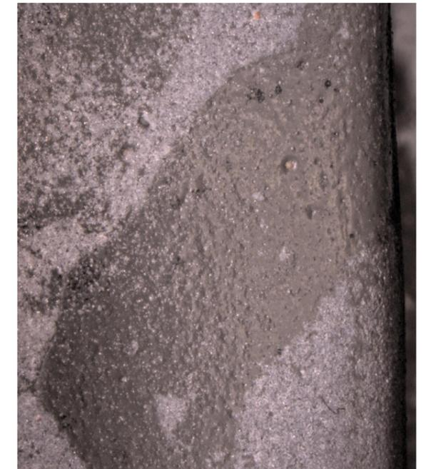
Figure 127 : Microscope image of the cast surface on the larger sized sample (contact). Ceramic sand mould coated with Crystalcast and Zirkofluid 6672. Part of the surface is transparent and part of it is more translucent.
