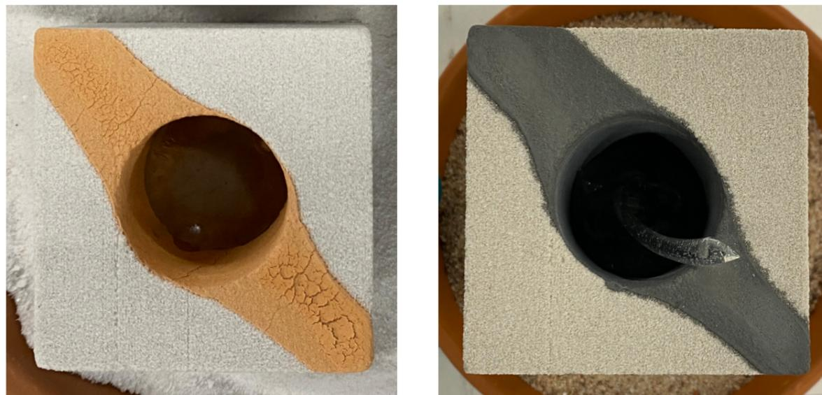
Figure 99 : Left Arkopal B 5 applied on quartz sand mould two times via flow application after the annealing schedule at 870°C.. Right same set up after hot pouring and annealing of glass. Colour difference is a clear indication of some kind of deterioration of the coating due to the prolonged exposure to high temperature.
