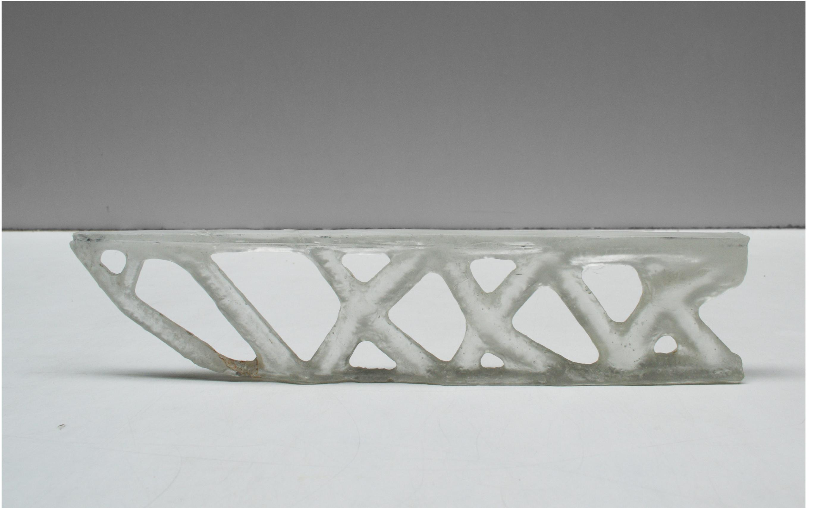
Figure 144 : Prototype after cutting the vent and glass tank using a diamond blade saw.
