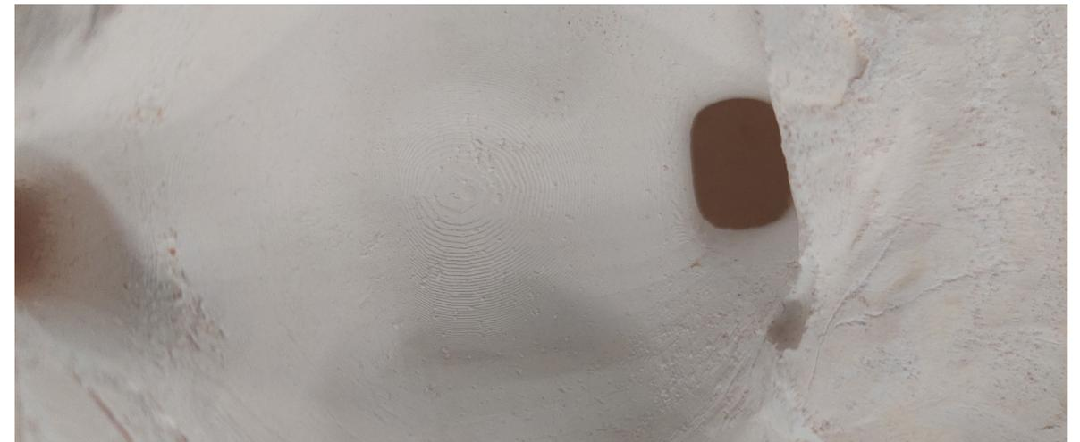
Figure 60 : Accuracy of the FDM printer is lower at around 1-2 mm which creates a visible pattern on the mould surface after the wax is burned off.
