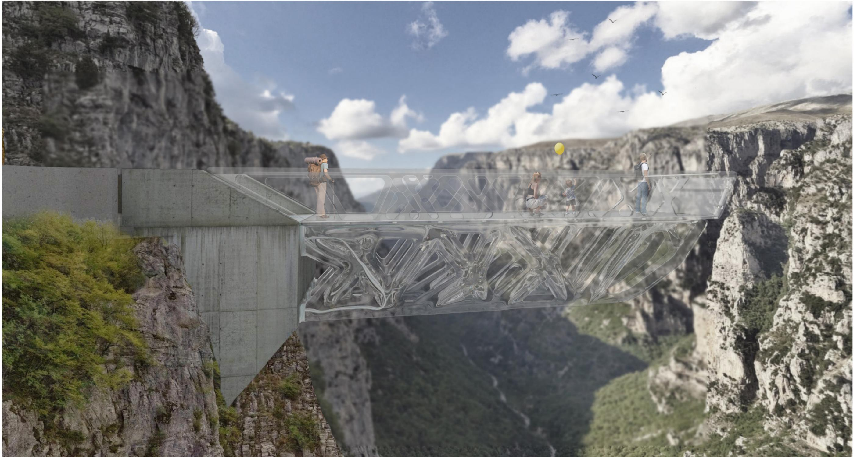
Figure 122 : Rendered view of the all glass bridge observatory. The two different fabrication methods are visible. Cast glass at the bottom and lamination of AWJ cut glass at the top.
