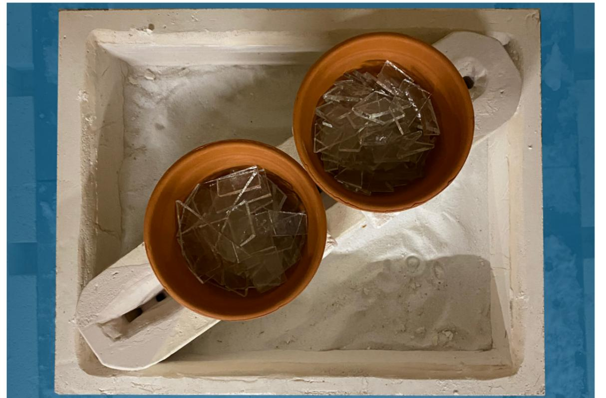
Figure 140 : Flowerpot set up inside the oven. Before firing.
