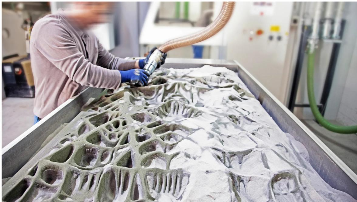
Figure 35 : Cleaning up the excess sand from the cured 3D printed sand moulds. This mould is used for the fabrication of prototype A.
