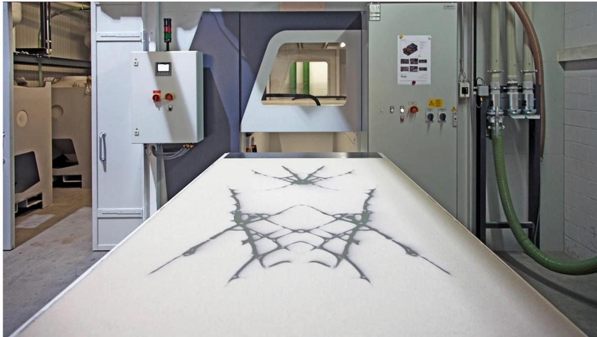
Figure 34 : 3D printed sand mould produces by binder jetting additive manufacturing method, Mould inside sand box, probably after drying.
