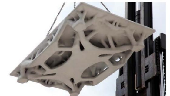
Figure 39 : Prototype B as realised (Jipa et al., 2016)
