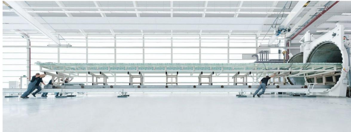
Figure 45 : Lamination of a 20 m.. long piece of float glass, <https://www.sedak.com/en/skills/laminating/>
