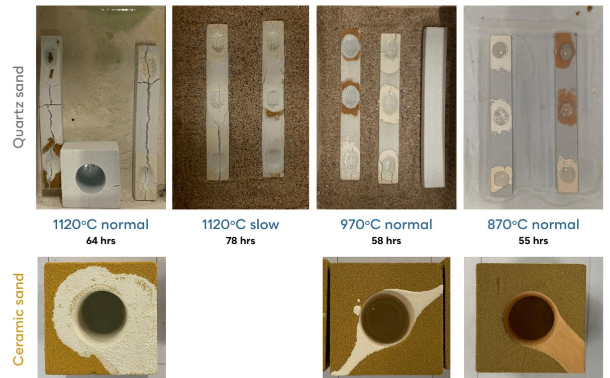
Figure 92 : Results for quartz sand moulds and different annealing schedules, 3DPS mould specimens after the firing schedule.
