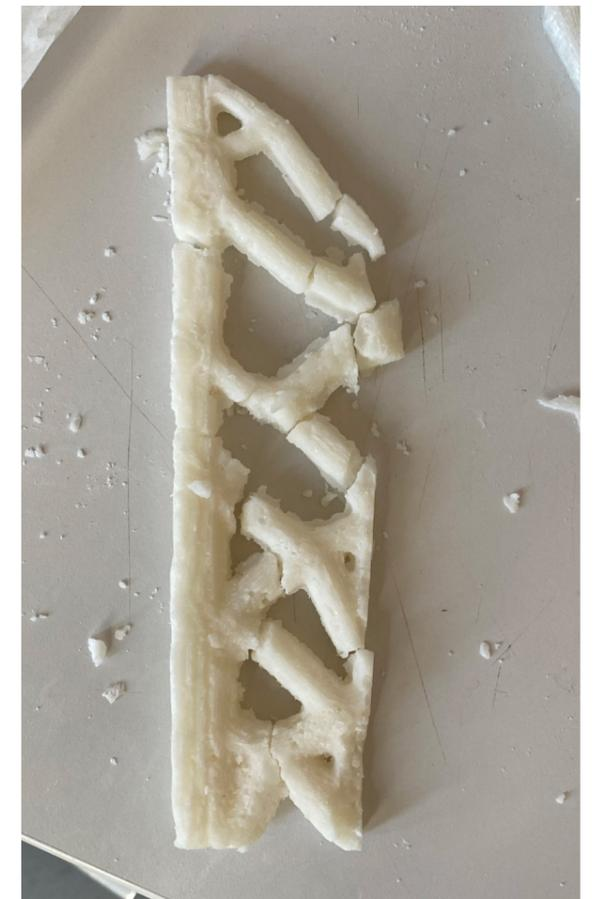
Figure 131 : Wax prototype after release from the PETG negative moulds. Geometry was scaled down 1:2 for this test to allow for quicker printing and to get some first impression of what needs to be improved. In this case the cross-sections are too small, thus the wax becomes fragile during separation.
