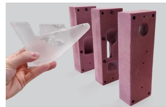
Figure 55 : Prototype of topologically optimized glass column. The prototype was produced using 3DPSM at the glass lab at TU Delft (Bhatia, 2019)
