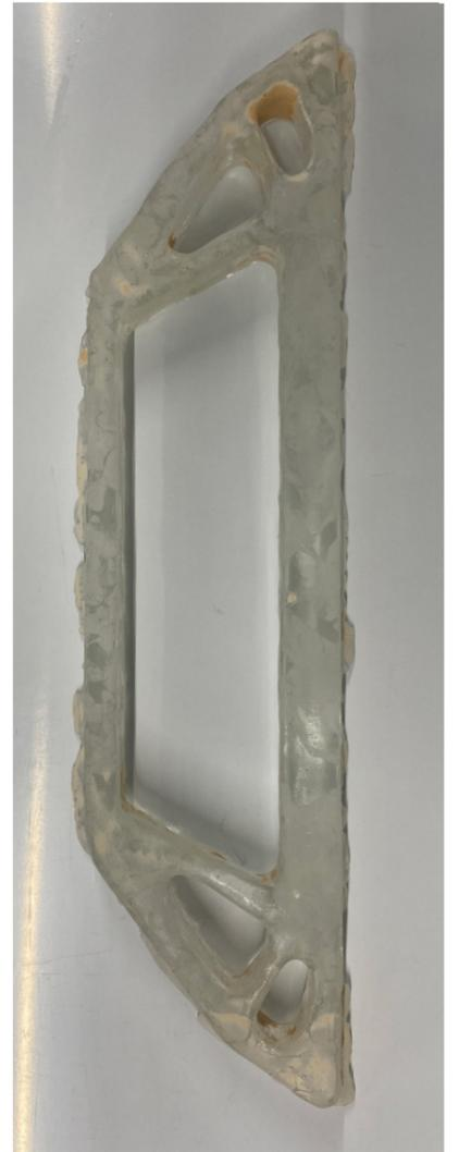
Figure 128 : From 3DPSM to cast glass component.
