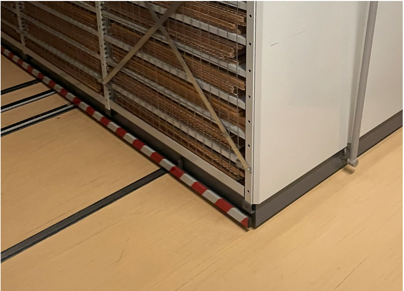
Figure 11: mobile compactor system for archive storage
