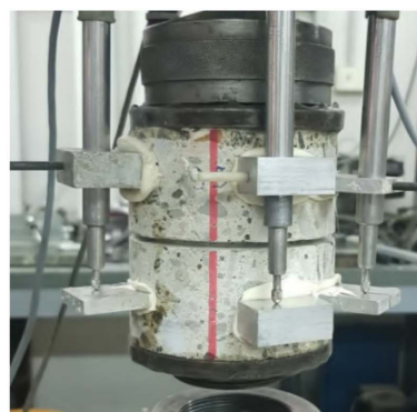
Fig. 4. Instrumentation for uniaxial tensile tests.
