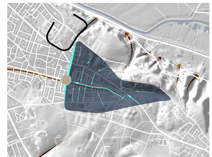
Image 9.14: Water catchment on the impenetrable surfaces of the valley crossing Broerdijk.
