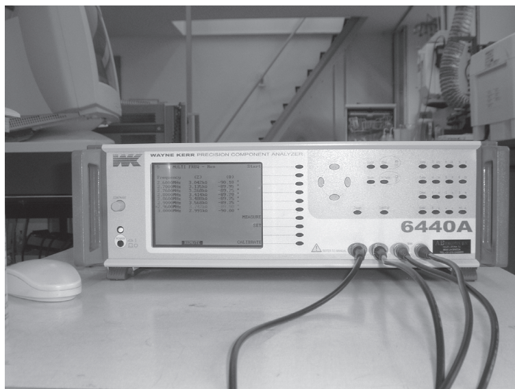
Figure D.2 The Network analyzer (Wayne-Kerr) used for impedance measurements.
