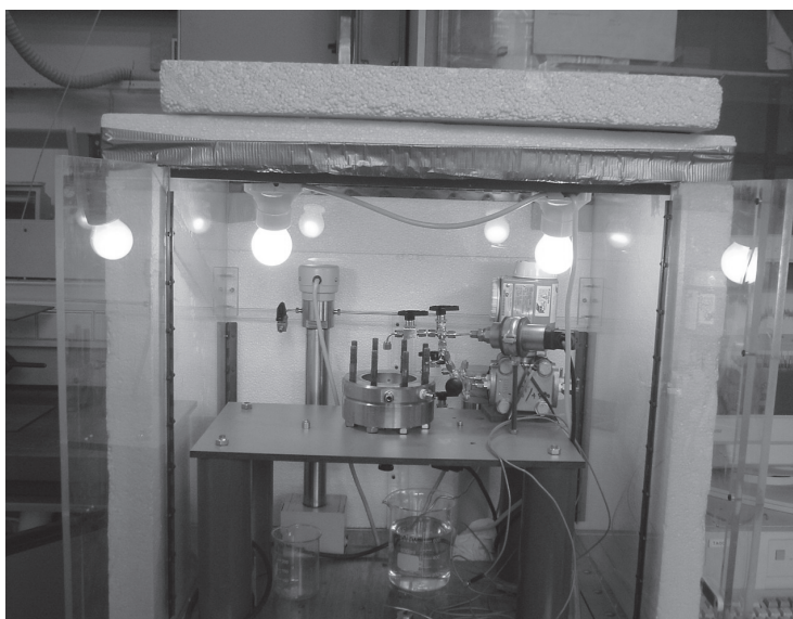
Figure D.1 Experimental set-up with high-pressure sample holder
