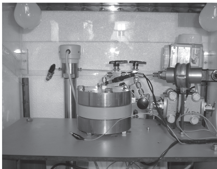
Figure D.4 The sample holder as parallel plate capacitor (with PEEK ring).
