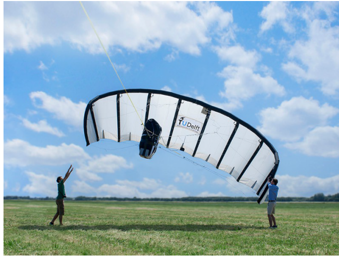
Figure 2.3: take off of the LEI kite V3 of the prototype developed at TU Delft [46]
