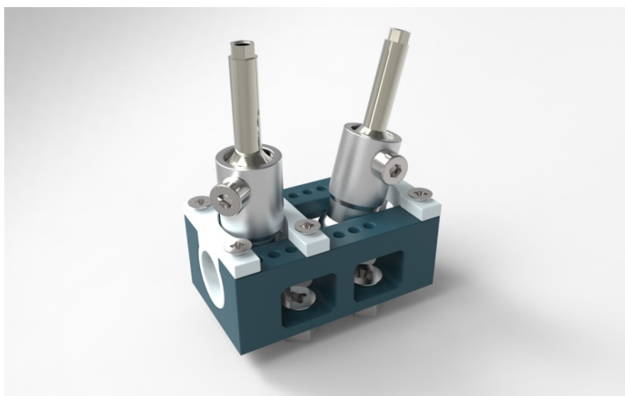
Figure 19: The optimized ball-joint concept. The working principle is identical to the concept explained in Figure 17, but was made smaller and detailed further. The abutments are attached to the holders by means of a screw that is inserted into the holder and clamps the abutment in place. The device can be attached to the prosthesis with screws that are positioned to fit to a standard prosthetic sleeve.
