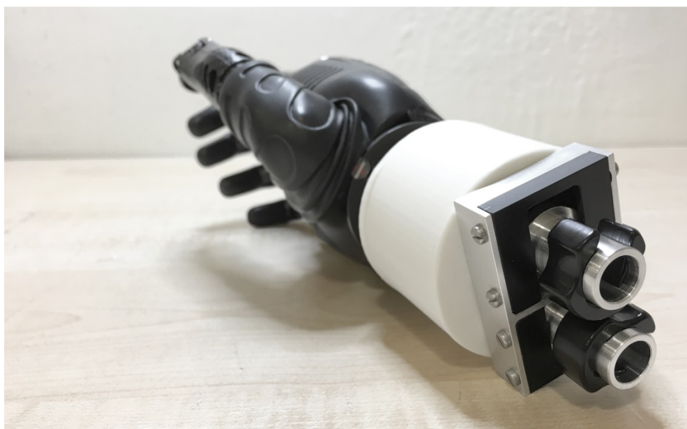
Figure 21: The machined prototype of the new attachment device attached to a prosthetic limb.
