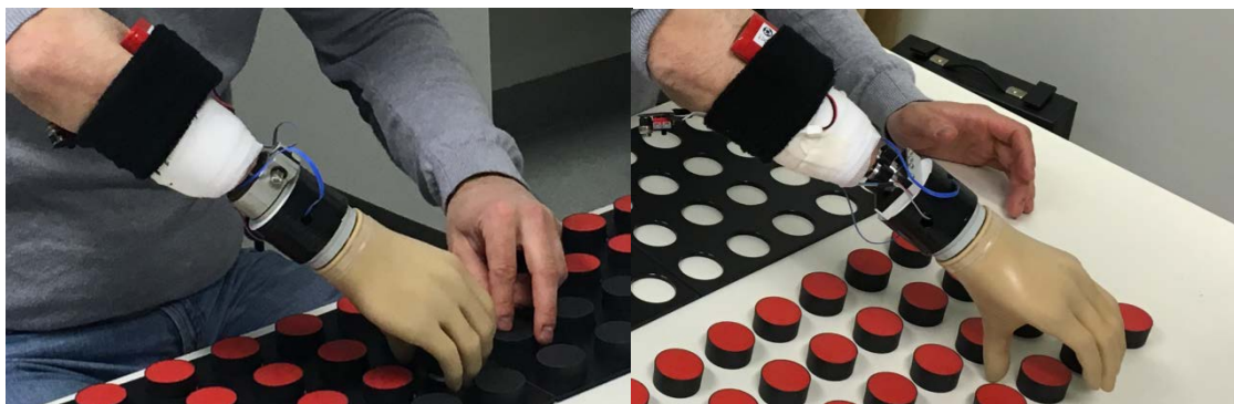
Figure 25: Setup of the prosthesis with the puck (left) and the Rotador (right)
