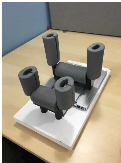
Figure 23: The rig that the patient placed his arm in for the analysis of the motion.
