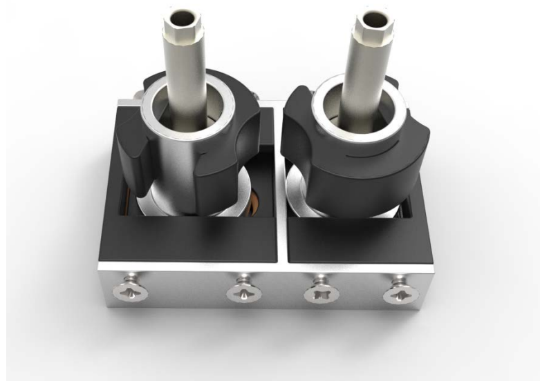
Figure 20: The flatter alternative for the ball joint concept. Plastic locks take the place of the screw attachment of the abutments, and the ball joint is replaced with a cylindrical holder (indirectly) placed on an elastic element.
