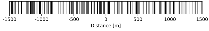
FIG. 4 Irregular distribution of \mathbf{x}_S^{(i)} along \mathbb{S}_0 . The black bars denote the positions of the sources.
