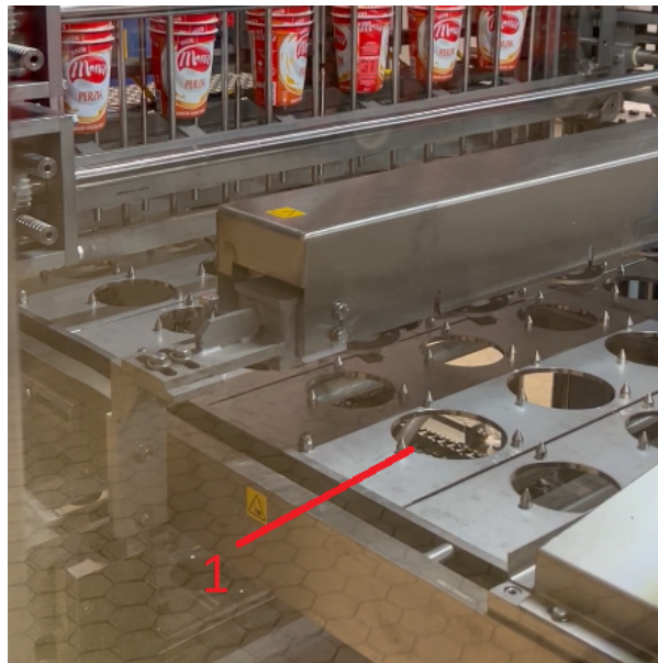
Figure 4.2: Chain with cup holes for transportation
