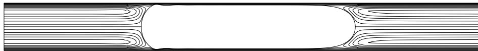
Figure 1.4: Streamlines in Taylor flow, revealing the circulation pattern in the liquid slug and the film layer between the bubble and the wall. Details of the numerical simulation are given in Chapter II.
