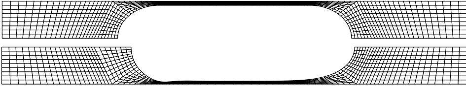
Figure 2.3: Example mesh. Top: initial mesh, bottom: converged mesh.
