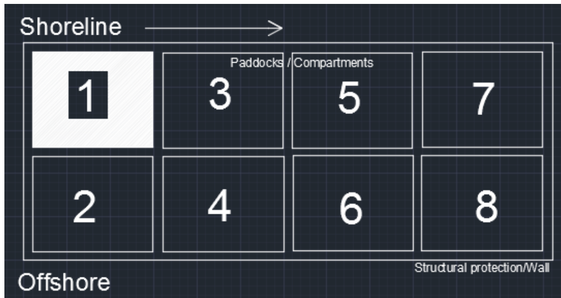
Figure 4-1 Placement of mud into compartments or 'paddocks' leading to section-by-section placement in compartments that would be relatively small compared to the dimensions required for simultaneous vertical or alongshore placement
