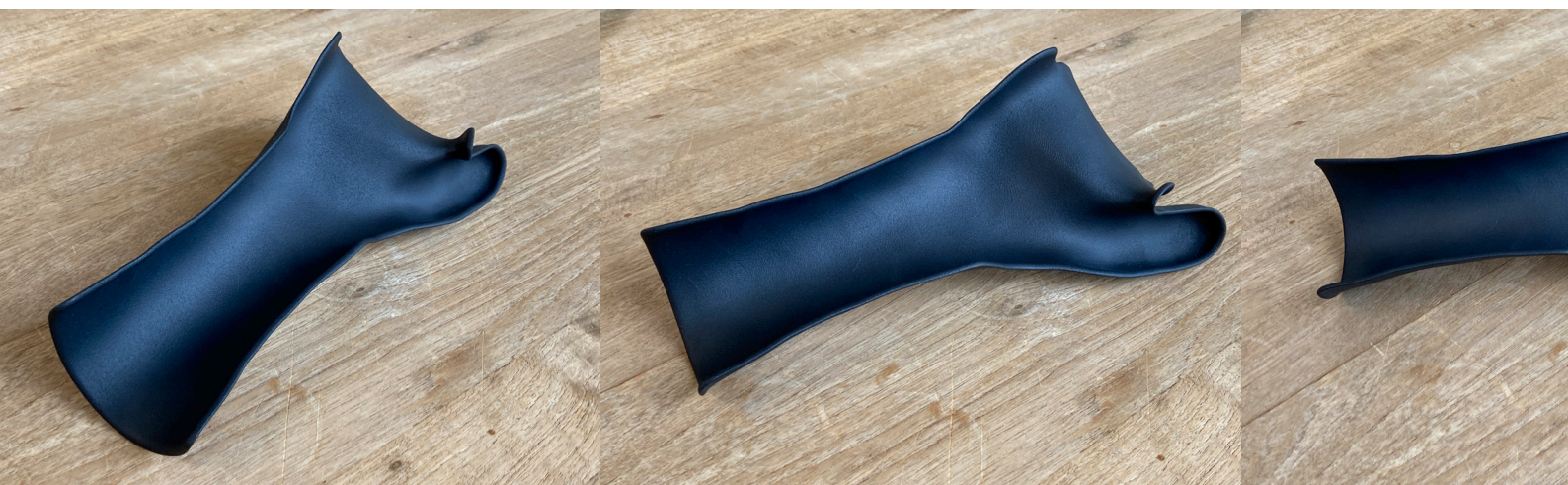
Figure 11: Overview of an orthosis directly from the 3D printer from various perspectives
