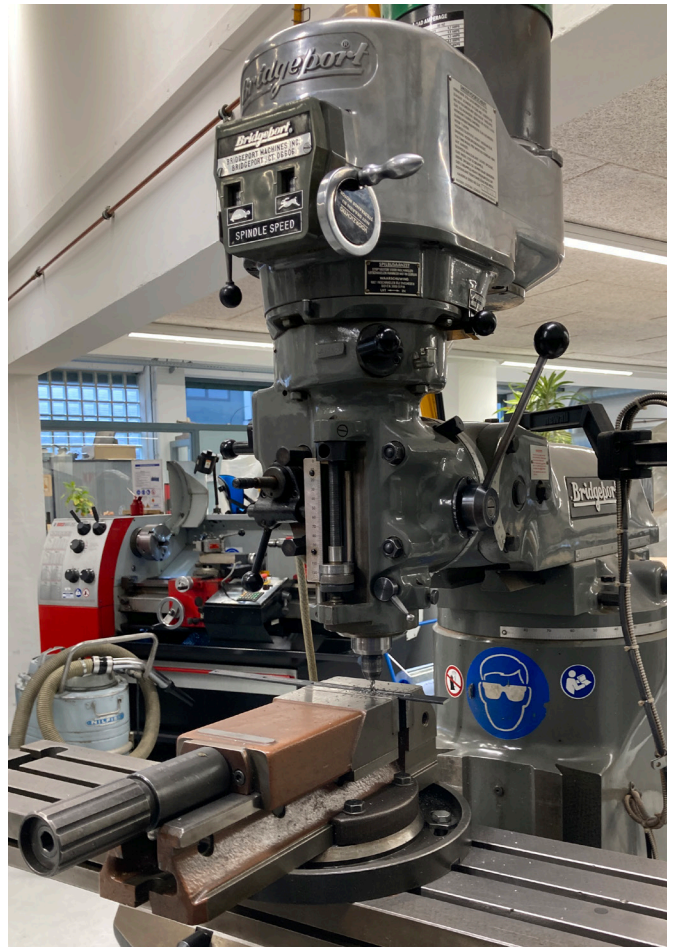
Figure 62: Milling the slots for the rod plate
