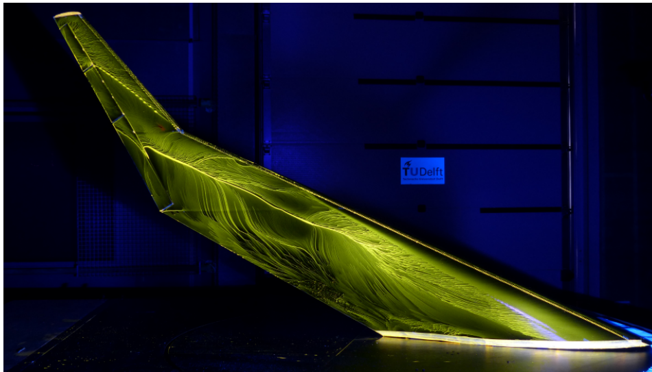
Figure 3.11: Windtunnel oil visualisation at \alpha = 22^\circ [8]
