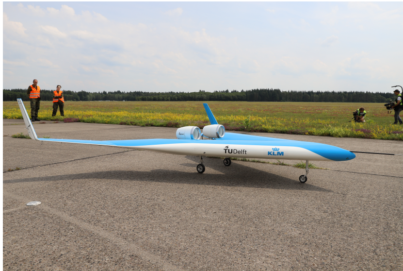
Figure 3.14: The scale flight test model of the Flying V in summer 2020. [22]
