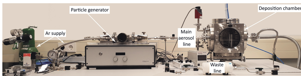
Figure 2.4: The experimental setup for dry aerosol direct writing (dADW)
