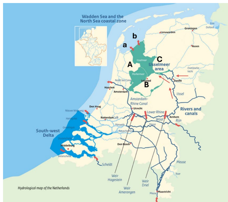
Figure 4.1 Hydrological Map of Netherlands (from Water Management in the Netherlands, Rijkswaterstaat, 2019). The main run-off toward IJssel Lake comes from Wieringermeer (A), Flevoland (B) and Nordoostpolder (C), while discharge control in Afsluitdijk is handled
