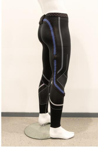
Figure 6.2: The pants with build-in IMU sensors [2].
