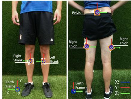
Figure 3.2: Sensor placement [2].
