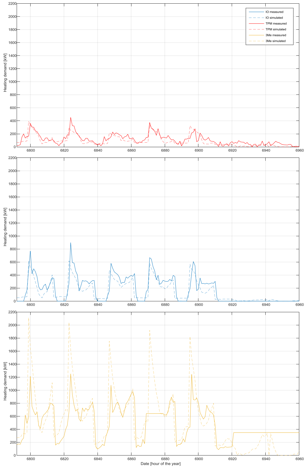
Figure 52 Measured & simulated heating demand TPM (above), IO (middle), and 3mE (below). Week period: 10 th – 16 th October 2016
