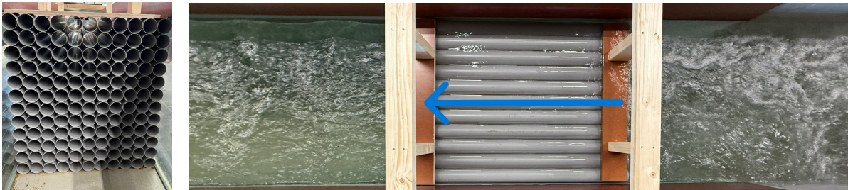
Figure 3.3: Flow conditioner, front view (left), top view (right)
