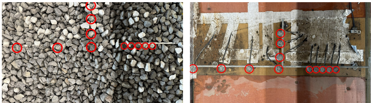
Figure 3.9: Upper pressure sensor array - Top view - marked - with rock layer (left) and after testing (right)
