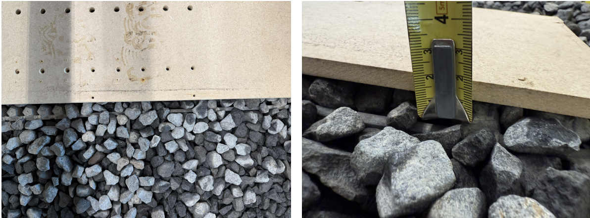
Figure 3.12: Layer thickness measurement, top view and side view of measurement
