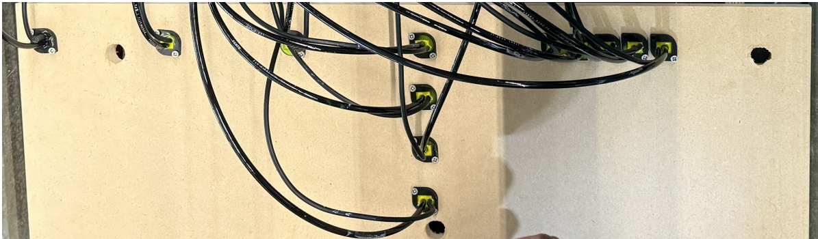
Figure 3.7: Lower Pressure Sensor Array underside - with reference tubes
