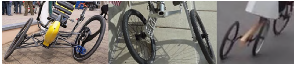
Figure 1.3: The three main categories of tilt mechanisms. From left to right: The parallelogram, the bell crank plus swing arm design, and the crank mechanism [32].
