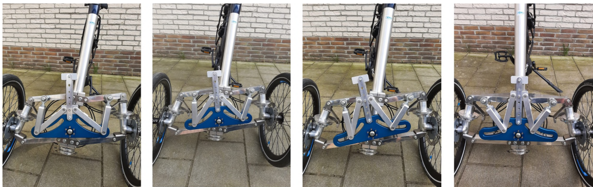
Figure 5.3: The tilt mechanism of the Dressel tilting tricycle for tie rod angles of 0%, 25%, 50% and 75%, respectively.
