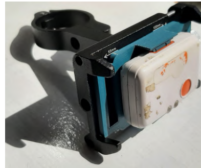
(b) The GUB Pro2 phone mount with the 3D printed clamp and the Shimmer3 IMU.
