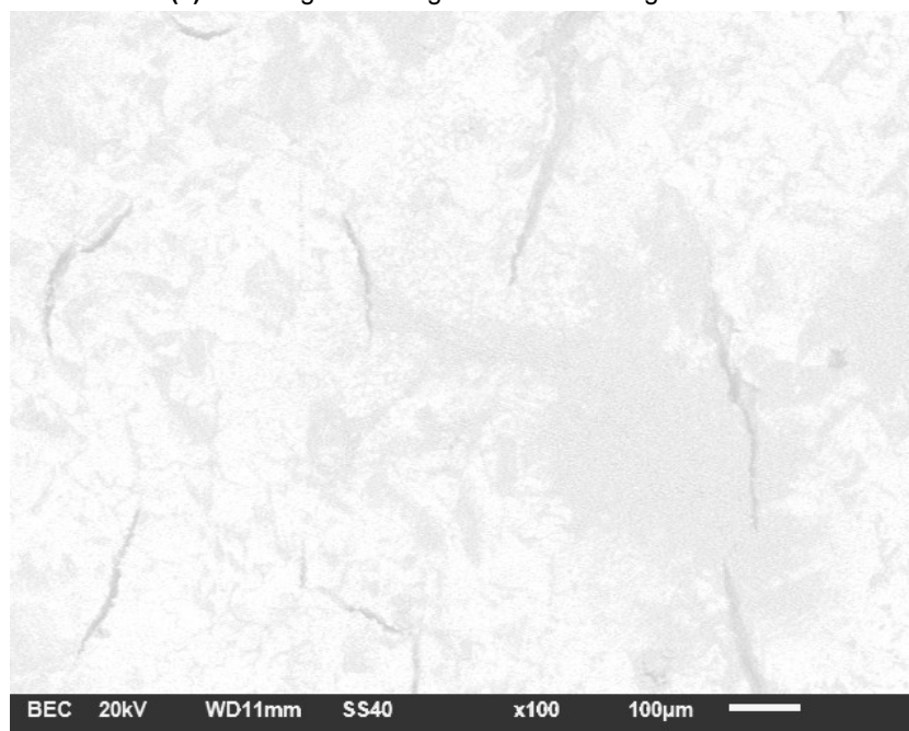
(b) BEC image of the Ag-GDE at 100x magnification (pt 1)
