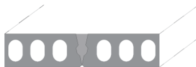
Figure 45: A prestressed hollow-core slabs
