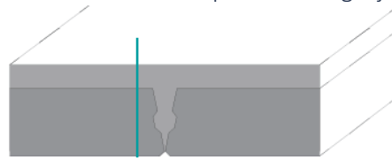
Figure 80: Sawing spot for prefab 2D components
