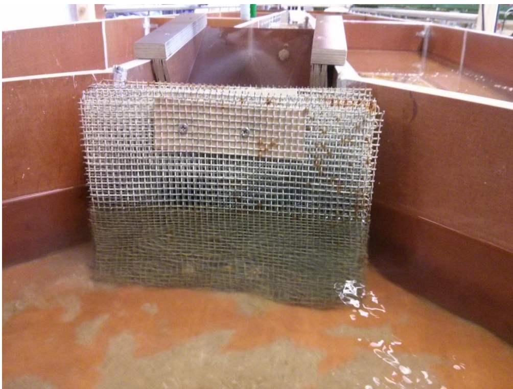
Figure H.18 – Ten steel grids attached to each other with a distance of 0.5 cm in between them to damp fluctuations in the water level from the area where the water flows into the flume.
