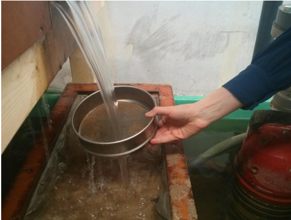
Figure H.21 – Sediment flowing out of the flume collected in a small sieve
