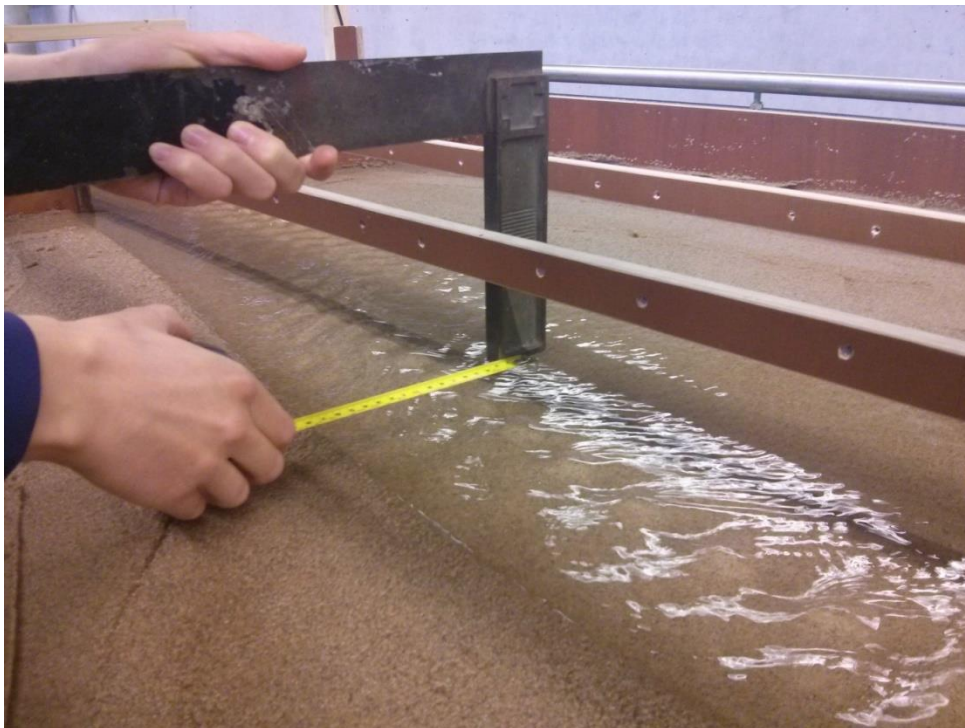
Figure H.22 – Measuring erosion rate with tapeline
