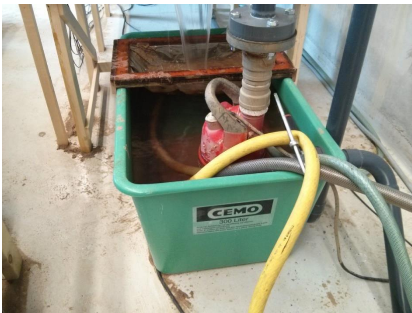
Figure H.10 – Water basin at downstream end of the flume. Green pipe is for water supply from the ball valve. Water that is sucked to the discharge pump flows through the yellow pipe. Water flowing out of the discharge pump goes through the brown pipe and lies in the water basin to keep any leakage of the connection to a longer green pipe (right in figure), that reaches up to the upstream end of the flume, inside the basin. The grey pipe (right in figure) attached to the water basin is used to drain water that exceeds a certain water level to prevent the basin from flooding and to keep the
