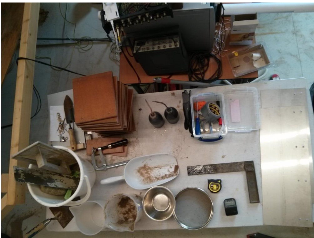
Figure H.6 – Tools used for measuring (e.g. small sieve, tapeline, stop watch, dye) and for preparing the bed and bank profile (e.g. chip, bucket, screwdriver).
