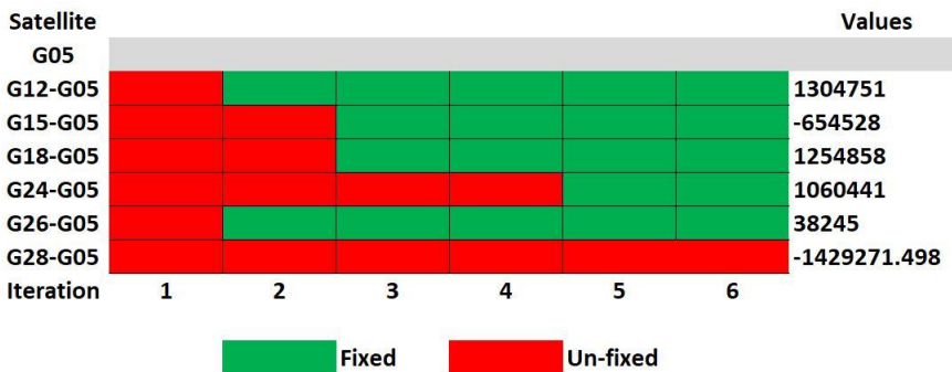
Figure 3.1: The subset ambiguities fixing (on the first GPS frequency) for a representative epoch, 00:30:00 on 17 July 2014 (DOY 198). The horizontal axis represents the consecutive EKF iterations, the vertical axis indicates the pair of GPS satellites for forming the double-differenced ambiguities.
